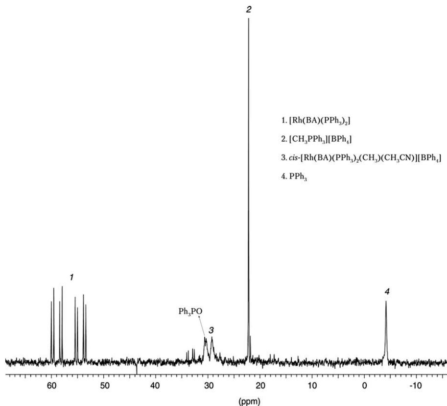
Fig. 2. The  $^{31}\text{P}\{^1\text{H}\}$  NMR ( $\text{CDCl}_3$ ) spectrum of the reaction mixture  $\{\textit{cis}\text{-}[\text{Rh}(\text{BA})(\text{PPh}_3)_2(\text{CH}_3)(\text{CH}_3\text{CN})][\text{BPh}_4] + \text{PPh}_3\}$  (1:1 mol) immediately after mixing of reactants.
