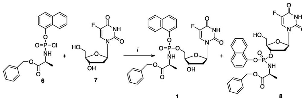
**Scheme 4.** Reagents and conditions: (i) tBuMgCl, dry THF, then phosphorochloridate (6), R.T., 16 h.
