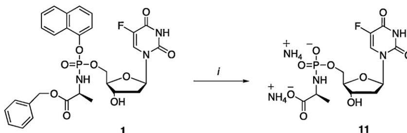
Scheme 5. Reagents and conditions: (i) Et<sub>3</sub>N:H<sub>2</sub>O (1:1), 35 °C, 16 h.
