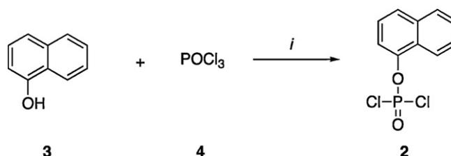
Scheme 1. Reagents and conditions: (i) dry Et<sub>2</sub>O, dry Et<sub>3</sub>N, –78 °C, 30 min then R.T., 3 h.
