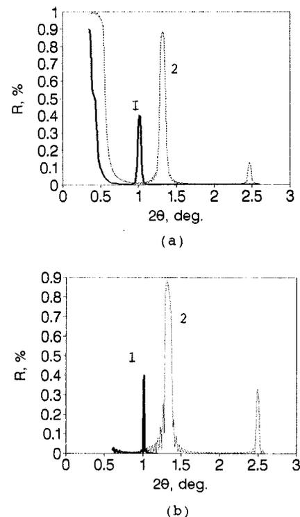
FIG. 1. (a) Experimental and (b) theoretical dependencies  $R=f(\Theta)$  for  $\lambda=1.54$  Å. (1) Multilayer carbon interference structure ( $N=118$ ,  $d=94$  Å); (2) Ni/C mirror ( $N=60$ ,  $d=72$  Å).
