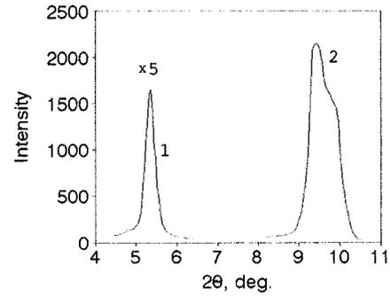
FIG. 2. Experimental dependencies  $R=f(\Theta)$  for  $\lambda=8.33 \text{ \AA}$ . (1) Multilayer carbon interference structure ( $N=118$ ,  $d=94$ ); (2) Ni/C mirror ( $N=60$ ,  $d=51 \text{ \AA}$ ).
