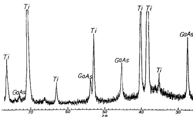
Fig. 9. X-ray diffraction pattern of an arsenic film on a gallium film electrodeposited on titanium substrate and annealed in N<sub>2</sub> at 300°C for 10 h. [Ga]/[As] = 49/51.
