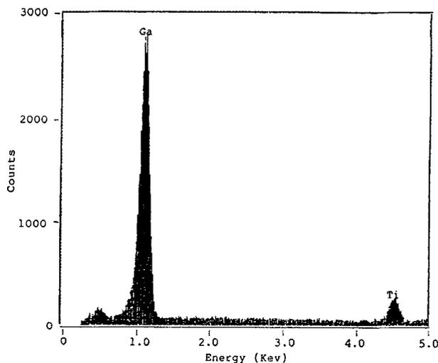
Fig. 21. EDS spectrum of Ga deposit with 30 mA/cm<sup>2</sup> from electrolyte at pH 2.5 containing 0.14M Ga(III).
