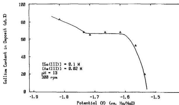
Fig. 4. Relationship between potential and gallium content in Ga/As films electrodeposited at 300 rpm from electrolyte at pH 13 containing  $0.1$  M Ga(III) and  $0.02$  M As(III).
