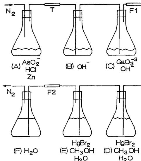
**Fig. 10. Schematic diagram of the experiment on arsine reaction.**
