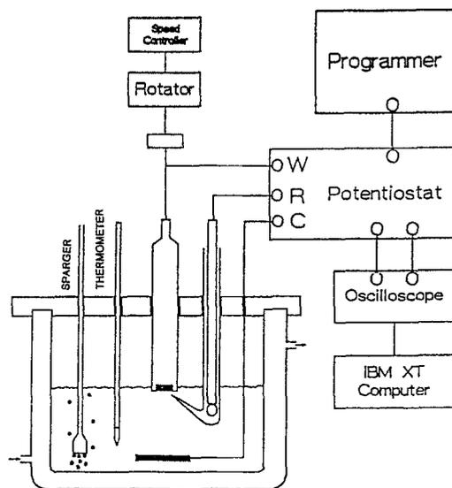
Fig. 1. Schematic diagram of the experimental apparatus and associated equipment.
