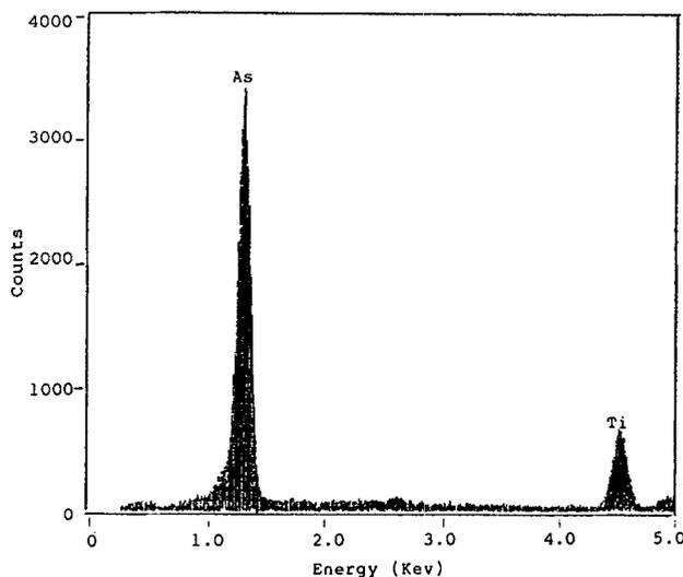
Fig. 22. EDS spectrum of As deposit with 30 mA/cm<sup>2</sup> from electrolyte at pH 2.5 containing 0.10M As(III).
