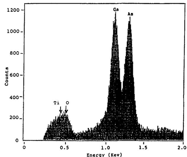
Fig. 20. EDS spectrum of a Ga/As film on titanium cathode, electrodeposited from electrolyte at pH 2.5 containing 0.14M Ga(III) and 0.10M As(III). [Ga]/[As] = 44.1/55.9 in the film.
