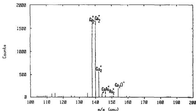
**Fig. 12. SIMS spectrum of a  $\text{GaAs}$  film electrodeposited at  $-1.67 \text{ V vs. Hg/HgO}$  from electrolyte at pH 13 containing  $0.1 \text{ M Ga(III)}$  and  $0.02 \text{ M As(III)}$ .**
