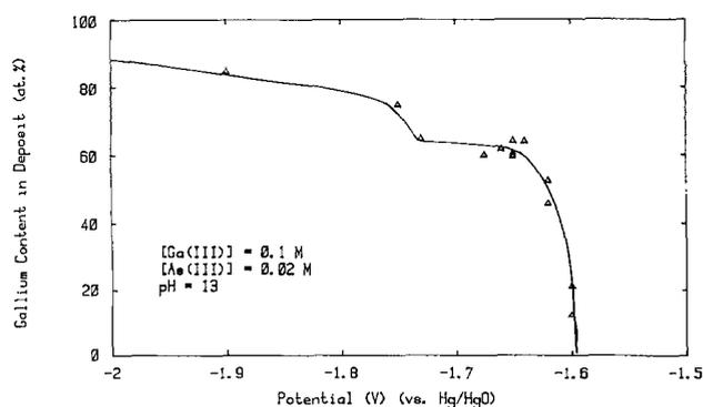
Fig. 2. Relationship between potential and gallium content in Ga/As films from electrolyte at pH 13 containing 0.1M Ga(III) and 0.02M As(III).
