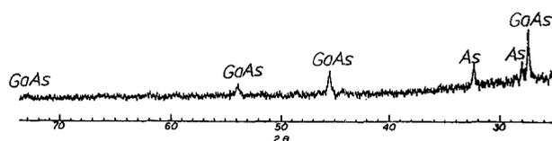
Fig. 7. X-ray diffraction pattern of a Ga/As film electrodeposited at -1.8 V vs. SCE from electrolyte at pH 13 containing 0.177M Ga(III) and 0.044M As(III), and annealed in nitrogen atmosphere at 300°C for 12 h. [Ga]/[As] = 39.0/61.0 in the film.
