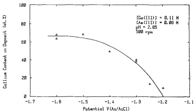
Fig. 15. Relationship between potential and gallium content in Ga/As films from electrolyte at pH  $2.85$  containing  $0.11M$  Ga(III) and  $0.08M$  As(III).
