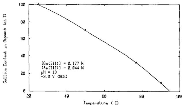
Fig. 3. Relationship between temperature and gallium content in Ga/As films electrodeposited at  $-2.0$  V vs. SCE from electrolyte at pH 13 containing  $0.177$  M Ga(III) and  $0.044$  M As(III).
