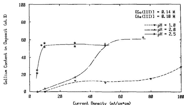
Fig. 16. Relationship between current density and gallium content in Ga/As films from electrolyte at 0.14M Ga(III) and 0.10M As(III) at pH 1.0, 2.0, and 2.5.
