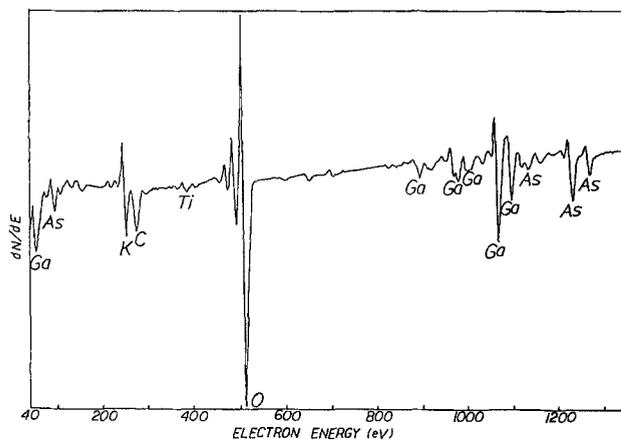
Fig. 13. Auger electron spectrum of a Ga/As film, on titanium cathode, electrodeposited at  $-1.62$  V vs. Hg/HgO from electrolyte at pH 13 containing  $0.1M$  Ga(III) and  $0.02M$  As(III).
