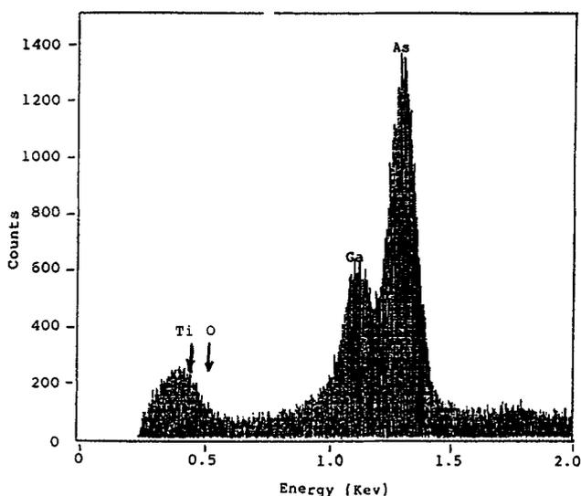
Fig. 19. EDS spectrum of a Ga/As film on titanium cathode, electrodeposited from electrolyte at pH 2.5 containing 0.14M Ga(III) and 0.10M As(III). [Ga]/[As] = 18.6/81.4 in the film.
