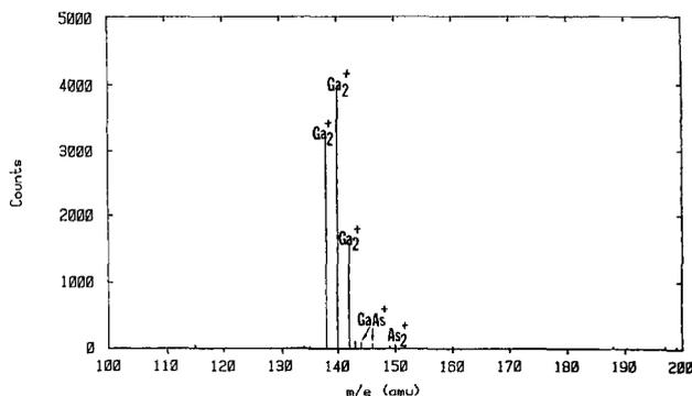
**Fig. 11. SIMS spectrum of standard gallium arsenide wafer.**
