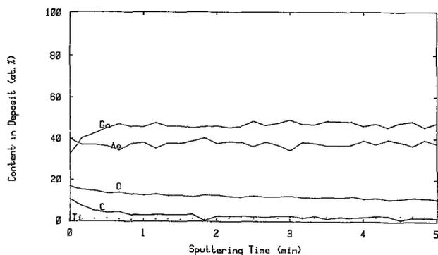
Fig. 14. Auger depth profile for a Ga/As film electrodeposited at  $-1.62$  V vs. Hg/HgO from electrolyte at pH 13 containing  $0.1M$  Ga(III) and  $0.02M$  As(III).
