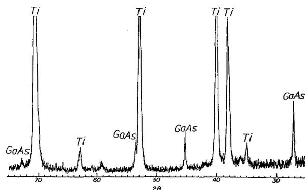
Fig. 8. X-ray diffraction pattern of Ga/As film on titanium substrate, electrodeposited at -1.67 V vs. Ag/AgCl from electrolyte containing 0.25M Ga(III), 0.05M As(III), and 2M KOH, and annealed in N<sub>2</sub> at 240°C for 21 h, [Ga]/[As] = 68.1/31.9 in the film.
