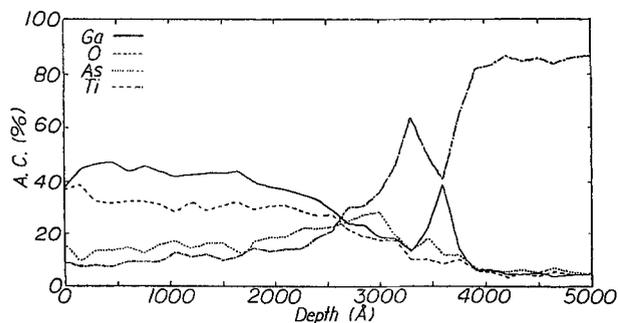
Fig. 18. Auger depth profile for a Ga/As film electrodeposited at 30 mA/cm<sup>2</sup> from electrolyte at pH 2.5 containing 0.14M Ga(III) and 0.10M As(III).
