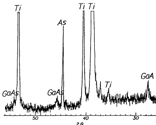
Fig. 17. X-ray diffraction pattern of a Ga/As film on titanium substrate, electrodeposited at 10 mA/cm<sup>2</sup> from electrolyte at pH 2.5 containing 0.14M Ga(III) and 0.10M As(III), and annealed at 260°C for 8 h.
