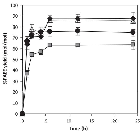
**Fig. 5.** Reactivity of CL-PCMC-lipase on biodiesel synthesis from FFAs and PFAD. The reactions contained 250 mg of FFAs or PFAD, 4:1 [EtOH]/[FFA] molar ratio, in the presence of 1:1 [*t*-BuOH]/[FFA] molar ratio with 20% (w/w) CL-PCMC-lipase. The reactions were incubated at 50 °C. Substrate: Palmitic acid (diamond); Oleic acid (square); Linoleic (triangle); and PFAD (circle).
