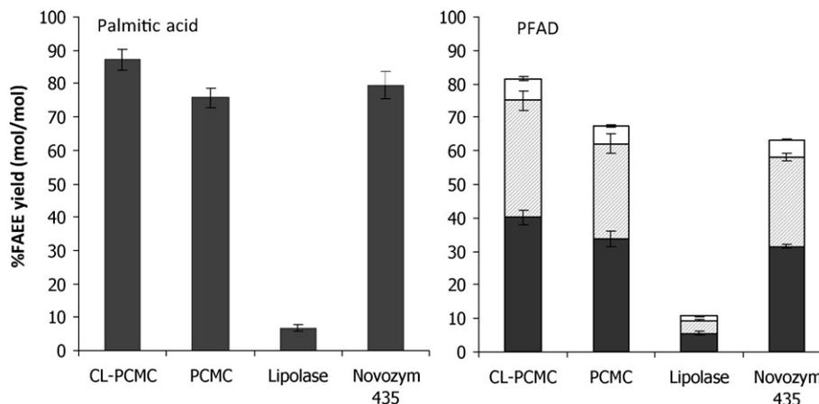
**Fig. 6.** Comparison of FAEE synthesis using different immobilized lipases. The reactions contained 250 mg of palmitic acid or PFAD, 4:1 [EtOH]/[FFA] molar ratio, in the presence of 1:1 [*t*-BuOH]/[FFA] molar ratio with 20% (w/w) CL-PCMC-lipase. The reactions were incubated at 50 °C for 6 h. CL-PCMC: CL-PCMC-lipase prepared from glycine in acetone; PCMC: PCMC-lipase prepared from glycine in acetone. FAEE products: ethyl palmitate (black); ethyl oleate (shaded); and ethyl linoleate (white).
