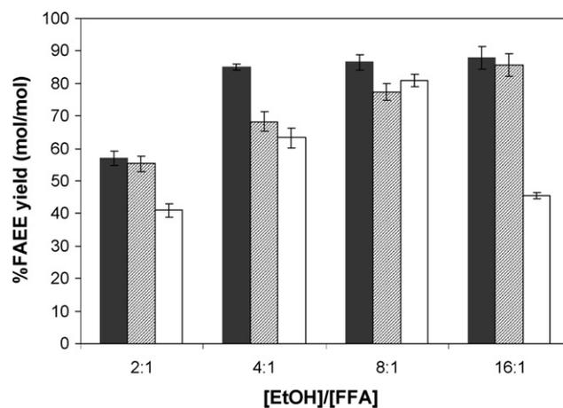
**Fig. 4.** Effects of nucleophile and co-solvent concentrations on FAEE synthesis. The reactions contained 250 mg of palmitic acid as the substrate with 20% (w/w) CL-PCMC-lipase with varying ethanol and *tert*-butanol ratios to FFA. The reactions were incubated at 50 °C for 6 h. [*t*-BuOH]/[FFA] = 1:1 (black); 2:1 (shaded); and 4:1 (white).
