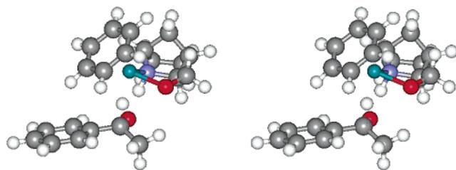
**FIGURE 2.** Favored TS showing a close contact between the methyl of the substrate and the amino alcohol oxygen and a tilted T-shaped arene-aryl interaction between catalyst and the phenyl group of the substrate (stereoimage).
