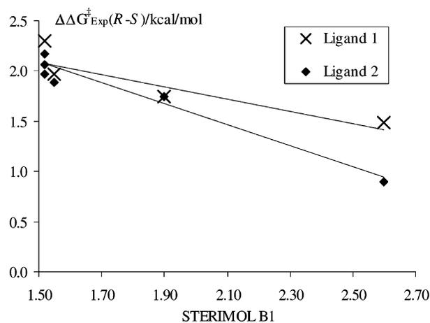
**FIGURE 6.** Correlation between  $\Delta\Delta G_{\text{Exp}}^{\ddagger}(R-S)$  (kcal/mol) and the STERIMOL B1 parameter of the alkyl group of the alkyl phenyl ketones Ru(*p*-cymene)(L). (L = 1: slope =  $-0.6$ ,  $R^2 = 0.77$ . L = 2: slope =  $-1.05$ ,  $R^2 = 0.94$ ).
