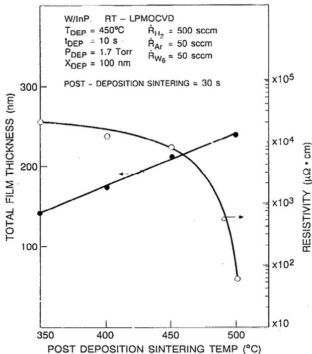
FIG. 1. RT-LPCVD W film thickness and resistivity as a function of the post-deposition sintering temperature.
