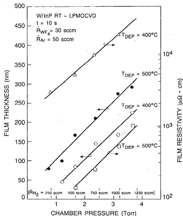
FIG. 2. RT-LPCVD W film thickness and resistivity as a function of the total chamber pressure and  $H_2$  flow rate during deposition.
