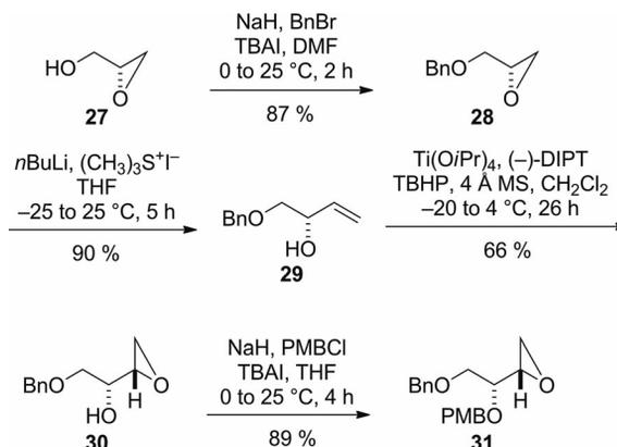
Scheme 4. Preparation of chiral epoxide **31**.
