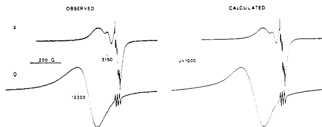
Figure 2. EPR spectra of the ortho-spin-labeled copper porphyrin V in toluene solution at room temperature. The X-band (9.11 GHz) spectrum is an 800 G scan obtained with 20 mW power and 0.63 G modulation amplitude. The Q-band (35.25 GHz) spectrum is a 1000 G scan obtained with 1.5 mW power and 2.5 G modulation amplitude. J is given in gauss. The simulated spectra include the contribution from "free" nitroxyl with a concentration 0.1% of the concentration of V.
