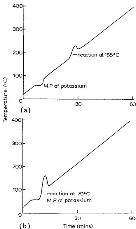
Fig. 1. Thermal analysis traces of liquid potassium-copper oxide reactions: (a)  $K + Cu_2O$ ; (b)  $K + CuO$ .
