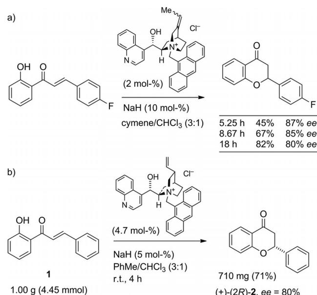
Scheme 5. Establishing optimal conditions for preparative applications of the reversible asymmetric catalytic 2'-hydroxychalcone to flavanone cyclization reaction. a) Analytical testing of a reaction for optimal yield vs. *ee* values by chiral HPLC. b) Preparative run of the reaction with 9-Am-CN-Cl and **1** for obtaining enantioenriched flavanone (+)-(2*R*)-**2**.
