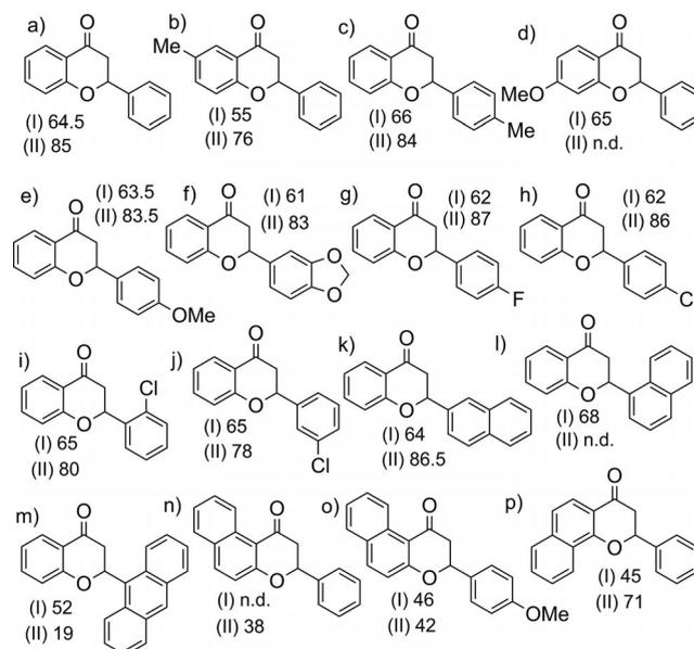
Figure 7. Intrinsic enantioselectivities (% *ee*) for the generation of substituted flavanones with two catalysts. Series I: 9-Am-CD-Cl/NaH (10 mol-%) in toluene/CHCl<sub>3</sub> (3:1). Series II: 9-Am-CN-Cl (5 mol-%) in cymene/CHCl<sub>3</sub> (3:1). Reaction conditions: hydroxy-chalcone (0.4 mmol) in solvent (4 mL), room temp. Analysis by chiral HPLC sampling of the reaction mixture; products were not isolated.
