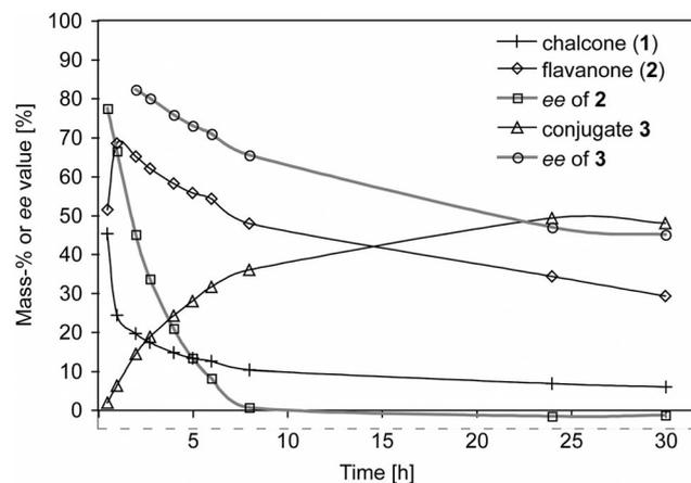
Figure 3. Kinetics and time-dependent enantioselectivity of chalcone/flavanone dimer **3** generation from 2-hydroxychalcone (**1**). Catalysis conditions: 9-Am-CN-Cl (9 mol-%), NaH (10 mol-%), toluene (4.5 mL/mmol), 45 °C. Internal standard for HPLC: 1,6-dibromo-2-isopropoxynaphthalene. Flavanone (**2**) was completely racemized after 8 h. The inverted ee ( $S > R$ ) of **2** after 10 h might be due to a kinetic resolution or a systematic integration error.
