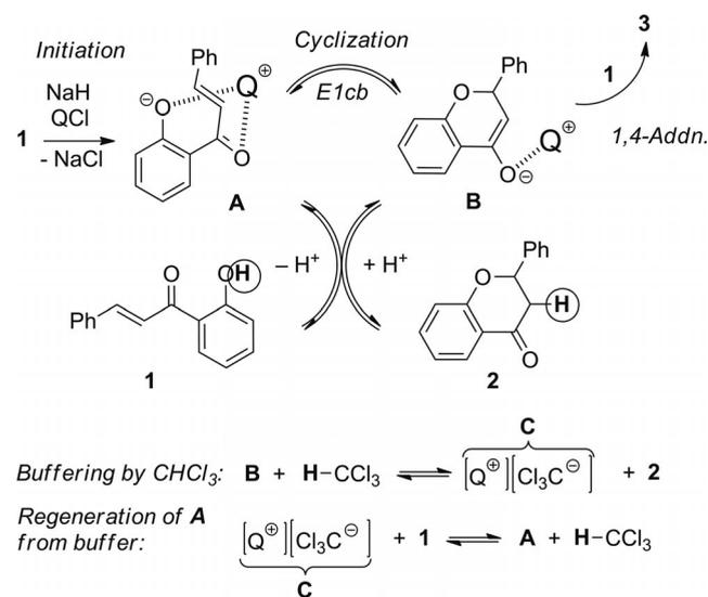
Scheme 3. Mechanism of the QCl/NaH-catalyzed cyclization of hydroxychalcones to flavanones: An asymmetric ion-pairing catalysis.
