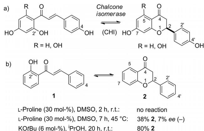
Scheme 1. a) Enzymatic cyclization of hydroxylated chalcones to flavanones. b) Attempted asymmetric catalytic cyclization of 2'-hydroxychalcones to flavanones.
