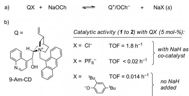
Scheme 4. a) The position of the ion-exchange equilibrium producing the catalyst resting state may depend on the nature of the counter-ion X<sup>-</sup>. b) The catalytic activity of 9-Am-CD-X salts in the **1** → **2** cyclization varies with the nature of X.
