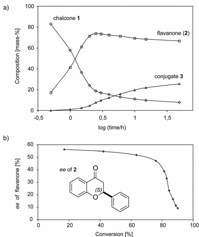
Figure 2. Course of the catalytic reaction **1**→**2** at 45 °C. Conditions: catalyst 9-Am-CN-Cl/NaH (10%), toluene (11 mL/mmol). Curves are interpolated to the measured values. a) Time-dependent composition of the reaction mixture. The data for **2** and **3** represent the sum of both enantiomers. Note the logarithmic timescale. b) Evolution of the enantiomeric excess of flavanone (**2**) as a function of the conversion of **1**.
