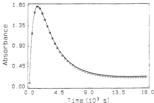
**Figure 2.** Response curves for combined (○) and indicator (—) reactions. First point at 10 s: initial acetoacetate concentration combined 3.02 mmol L<sup>-1</sup>, indicator 4.72 mmol L<sup>-1</sup>; pH 8.60, 25 °C, 0.49 mol L<sup>-1</sup> glycine, and 8.3 mmol L<sup>-1</sup> nitroprusside.
