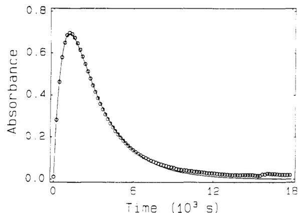
**Figure 6.** Experimental (○) and calculated (—) response curves of the combined reaction. One absorber, pH 8.6, 25 °C, 0.492 mmol L<sup>-1</sup> acetoacetate, 0.667 mol L<sup>-1</sup> glycine, and 8.3 mmol L<sup>-1</sup> nitroprusside.
