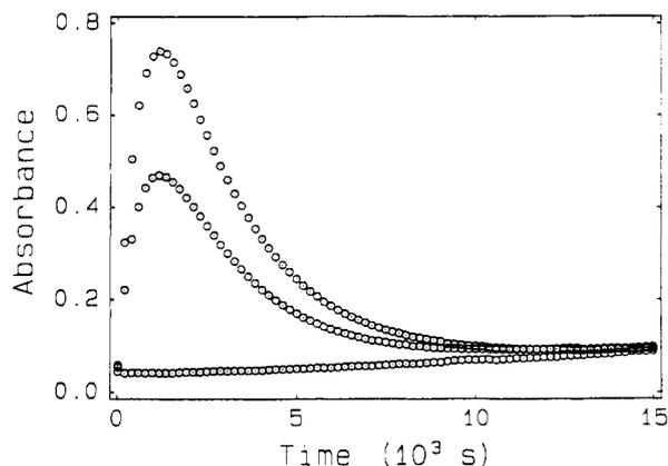
**Figure 1.** Response curves for combined (top), indicator (middle), and blank (bottom) reactions: pH 8.60, 25 °C, 0.67 mol L<sup>-1</sup> glycine, 1.18 mmol L<sup>-1</sup> acetoacetate, and 8.3 mmol L<sup>-1</sup> nitroprusside.
