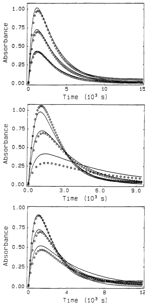
**Figure 7.** Experimental ( $\odot$ ) and calculated (—) response curves of the combined reaction. All frames: pH 8.6, 25 °C, multiple data sets (11 runs, 1005 points); fixed concentrations are at level 2 in Table I. (A, top panel) Acetoacetate (bottom to top): 0.295, 0.492, 0.688 mmol  $\text{L}^{-1}$ . (B, middle panel) Glycine (bottom to top): 0.333, 0.667, 1.00 mol  $\text{L}^{-1}$ . (C, bottom panel) Nitroprusside (bottom to top): 4.15, 8.30, 16.6 mmol  $\text{L}^{-1}$ .
