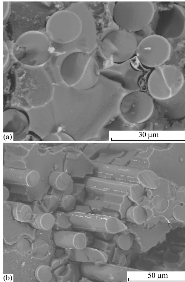
Fig. 5. Fracture surfaces of SiC/SiC composites: (a) no interphase, (b) three-layer interphase.
