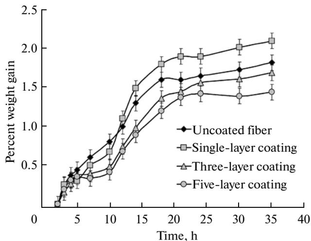
Fig. 4. Weight gain as a function of fiber oxidation time.
