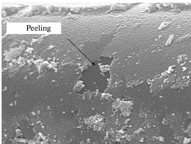
Fig. 3. Peeling of the outermost layer in a multilayered coating.
