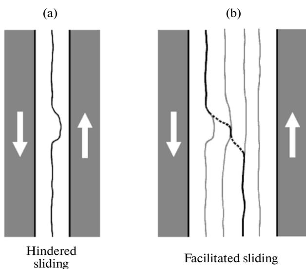
**Fig. 8.** Schematic illustrating fiber sliding relative to the matrix: (a) sliding hindered by an asperity; (b) a change in sliding plane to obviate an asperity.
