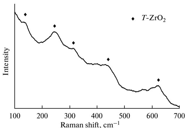
Fig. 2. Raman spectrum of the surface of a coated fiber.
