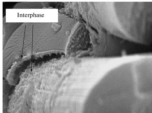
Fig. 6. Interphase delamination upon fracture of the composite.
