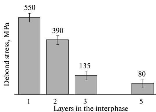
**Fig. 7.** Fiber debond stress in the composite against the number of  $\text{ZrO}_2$  layers in the interphase.
