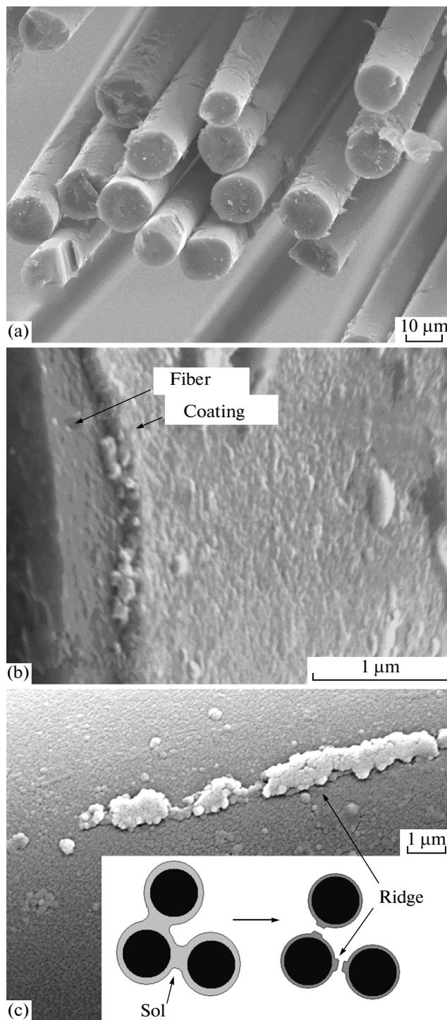
**Fig. 1.** Coated fibers: (a) general view of a fiber tow, (b) surface of an individual fiber, (c) surface ridge and schematic illustrating ridge formation.
