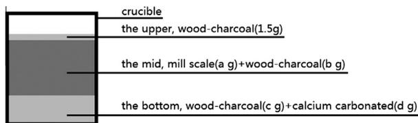
Fig. 3. Diagram of crucible filling.
