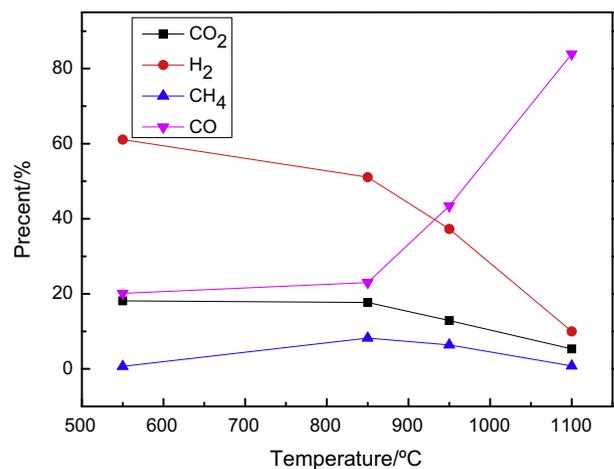
Fig. 5. Gas compositions of combination distribution of wood-charcoal by microwave heating (volume percent).
