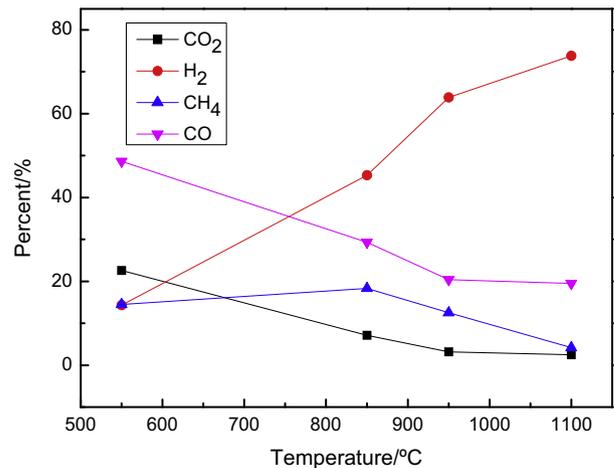
Fig. 4. Gas compositions of wood-charcoal by microwave heating (volume percent).
