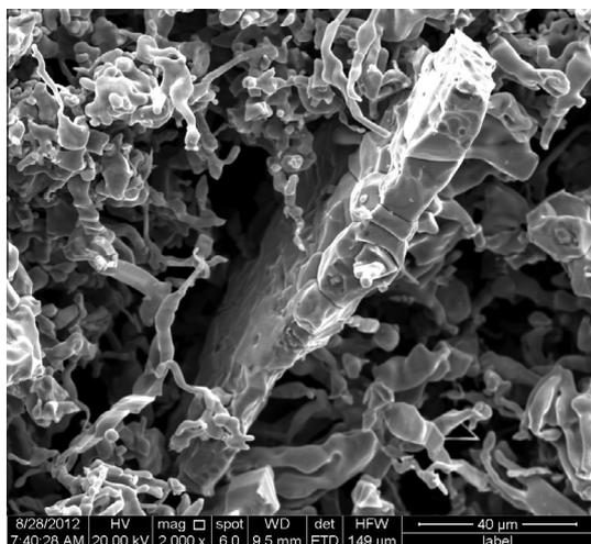
Fig. 7. SEM of reduced iron powder of 5 min for holding time at 1150 °C.
