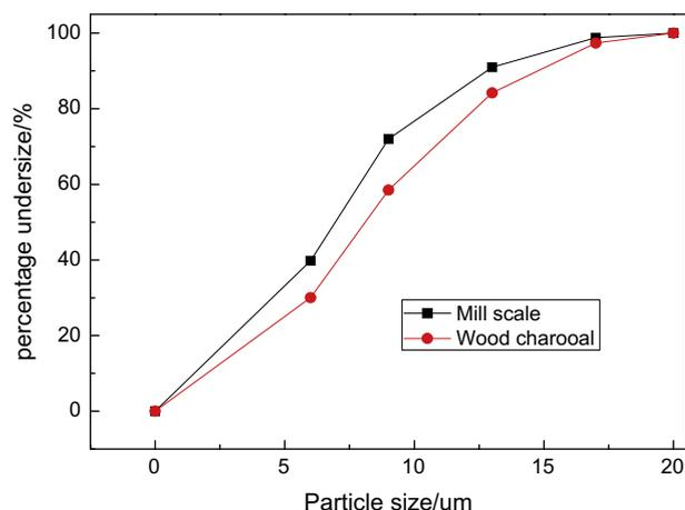
**Fig. 1.** Particle size distributions of mill-scale and wood-charcoal.
