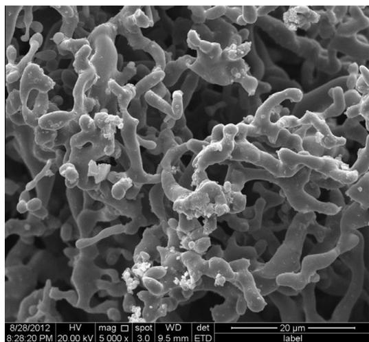
Fig. 8. SEM of reduced iron powder of 50 min for holding time at 1150 °C.
