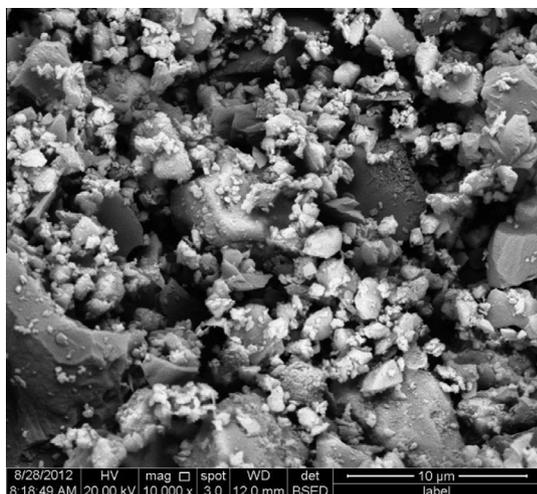
Fig. 6. SEM of the mixture of wood-charcoal and mill-scale.
