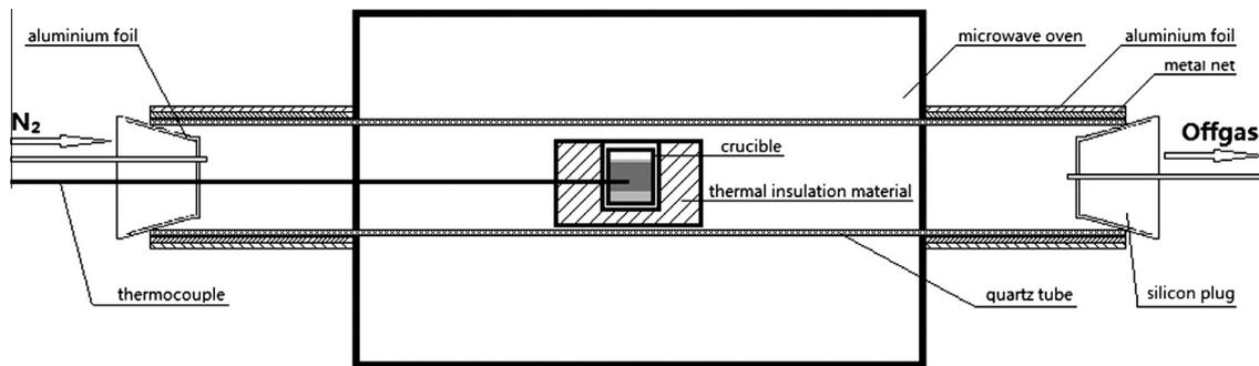
Fig. 2. Diagram of microwave tube furnace.
