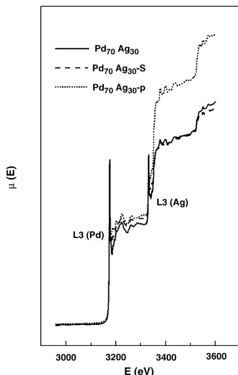
Fig. 4. XANES for the L3 edge of Ag in three  $\text{Pd}_{70}\text{Ag}_{30}$  samples heated to 250 °C in air. The L3 edges for Pd and Ag are at 3173 and 3351 eV, respectively.
