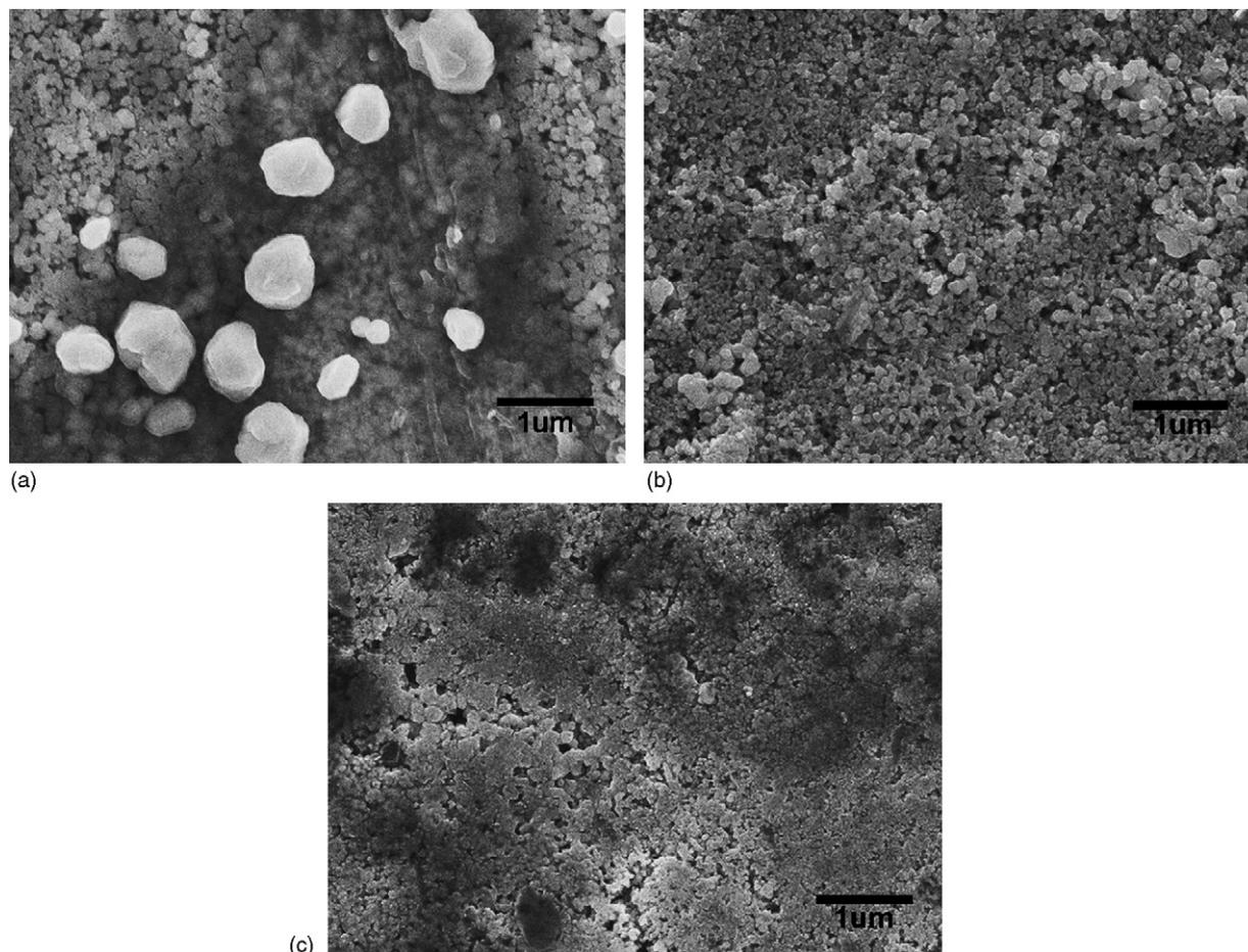
Fig. 1. SEM micrographs of three Pd<sub>70</sub>Ag<sub>30</sub> nanoparticle pellets after heating in air at 250 °C: (a) Pd<sub>70</sub>Ag<sub>30</sub>, (b) Pd<sub>70</sub>Ag<sub>30</sub>-s, and (c) Pd<sub>70</sub>Ag<sub>30</sub>-p.
