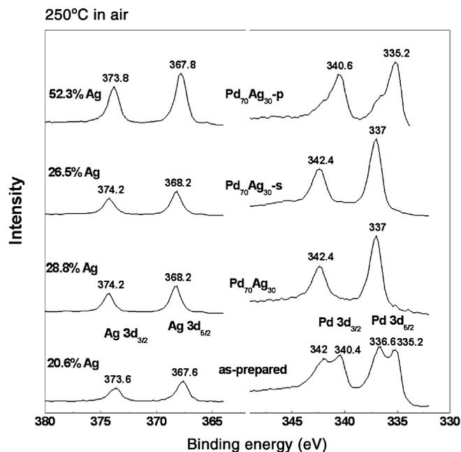
Fig. 3. The Ag (3d<sub>3/2</sub> and 3d<sub>5/2</sub>) and Pd (3d<sub>3/2</sub> and 3d<sub>5/2</sub>) peaks from ESCA analysis for various Pd<sub>70</sub>Ag<sub>30</sub> samples before and after heating at 250 °C. The surface composition of Ag (excluding the oxygen content) in each sample is shown on the curve.
