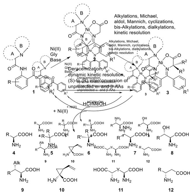
As shown in Scheme 1, generically represented tridentate ligands (*S*)- or (*R*)-1 are reacted with glycine and a source of Ni(II) ions to produce Schiff base complex 2, serving as a versatile chiral nucleophilic glycine equivalent. Square-planar Ni(II) complex 2 readily reacts with various electrophilic reagents to afford products 3 with usually high chemical yields
