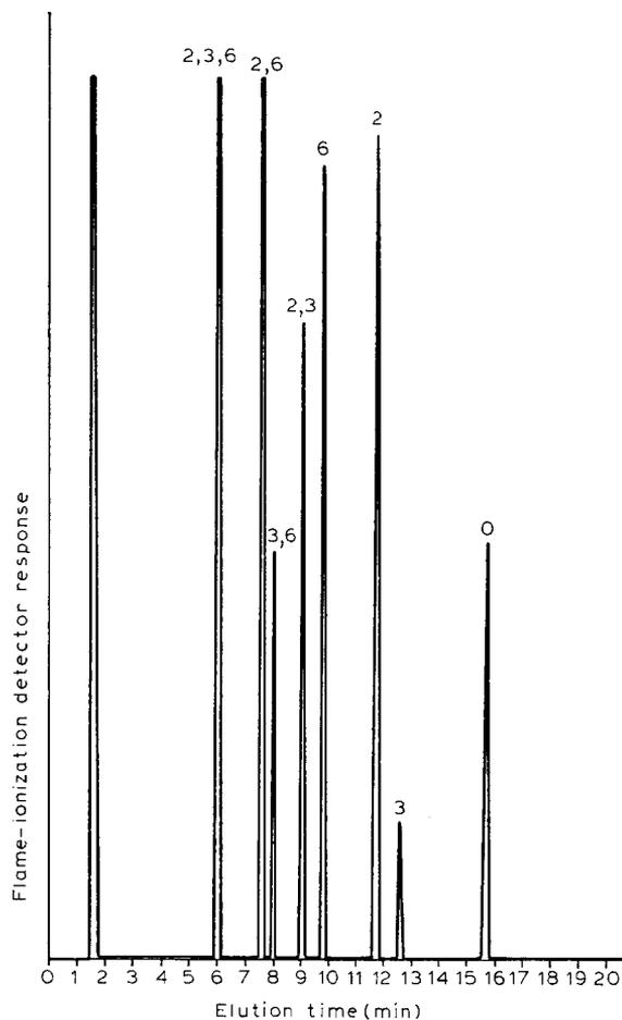
Fig. 1. G.I.c. chart of separation of partial ethylated alditol acetates obtained from *O*-ethylcellulose by hydrolysis, reduction, and acetylation. The numbers indicate the positions of the ethyl groups.
