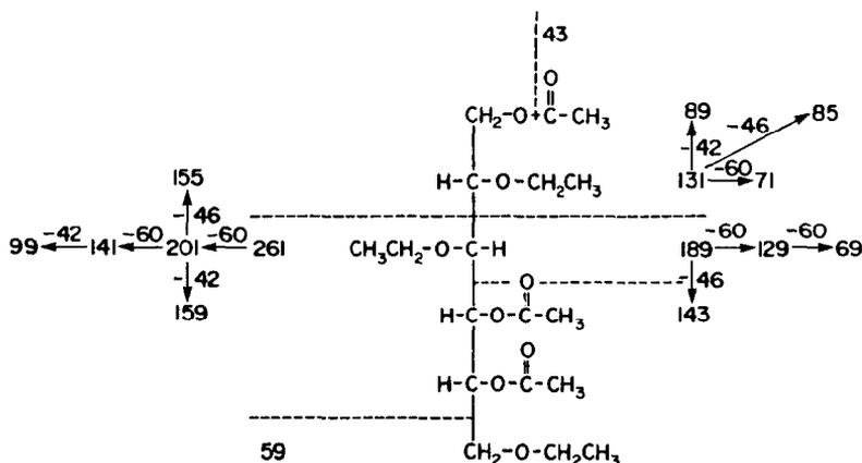
Fig. 2. The origin of the major fragment-ions obtained from e.i.-mass spectrometry of 1,4,5-tri-*O*-acetyl-2,3,6-tri-*O*-ethyl-D-glucitol.
