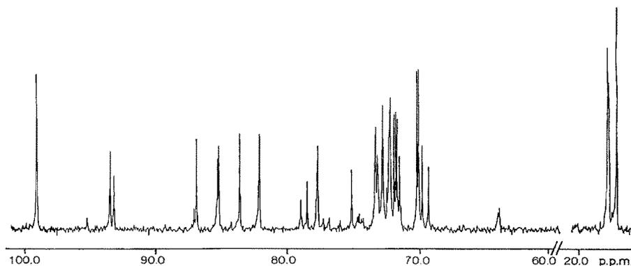
Fig. 4. 400-MHz,  $^{13}\text{C}$ -n.m.r. spectrum of hydrolyzed *O*-ethylcellulose (d.s. 2.3) in  $\text{D}_2\text{O}$ , recorded at  $21^\circ$ . Chemical-shift values are relative to internal acetone ( $\delta$  31.4).
