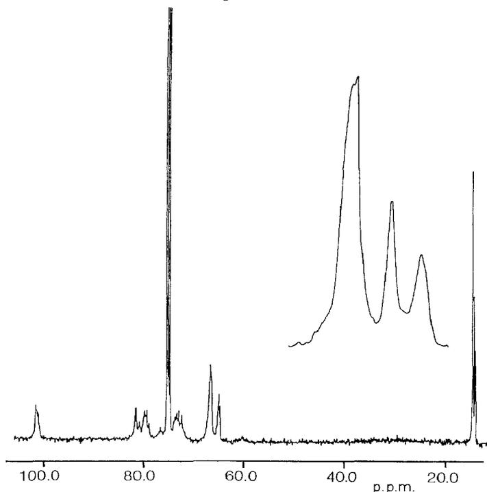
Fig. 3. 400-MHz,  $^{13}\text{C}$ -n.m.r. spectrum of *O*-ethylcellulose (d.s. 2.3) in  $\text{CDCl}_3$ , recorded at  $21^\circ$ . Chemical-shift values are relative to internal acetone ( $\delta$  31.4).
