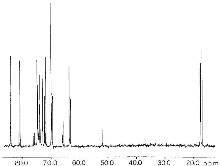
Fig. 5. 400-MHz,  $^{13}\text{C}$ -n.m.r. spectrum of hydrolyzed and reduced *O*-ethylcellulose (d.s. 2.3) in  $\text{D}_2\text{O}$ , recorded at  $21^\circ$ . Chemical-shift values are relative to internal acetone ( $\delta$  31.4).
