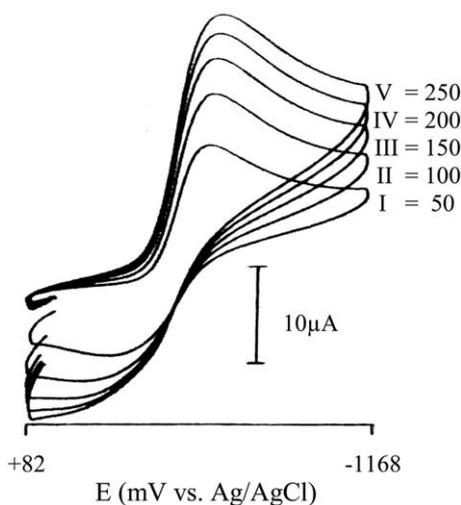
Fig. 4. Cyclic voltammogram of (1), 10<sup>-3</sup> M in dichloromethane shows Mn(III/II) couple in the range of 82 to –1168 mV, between scan rates of 50–250 mV s<sup>-1</sup> (I–V).
