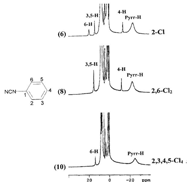
Fig. 2.  $^1\text{H}$  NMR spectra of manganese(III)porphyrin complexes: TPPMn(2,3,4,5-Cl<sub>4</sub>pcyd) (10), TPPMn(2,6-Cl<sub>2</sub>pcyd) (8), and TPPMn(2-Clpcyd) (6), in  $\text{CDCl}_3$  at 300 K.
