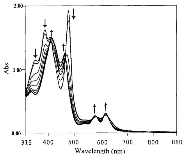
Fig. 5. Optically transparent thin-layer electrode cell electronic spectra of (1) (0.1 M TBAH electrolyte) in dichloromethane. Potential range for forward reaction –0.7 to –1.2, for backward reaction –0.3 to +0.2 V vs. Ag/AgCl reference electrode.
