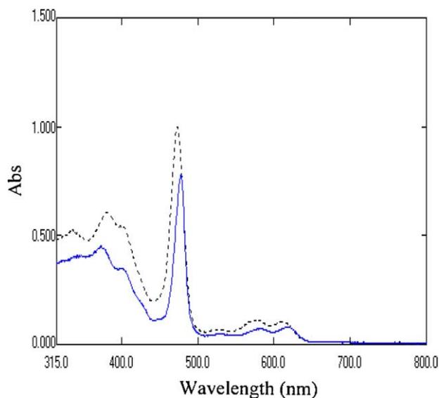
Fig. 1. UV–Vis spectra of TPPMnCl (—) and TPPMn(4-Mepcyd) (---),  $1.25 \times 10^{-5} \text{ M}$  in dichloromethane.
