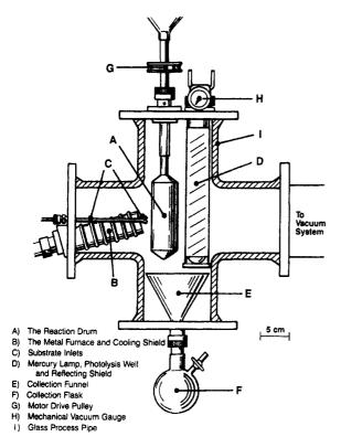
Figure 1. Photochemical metal vapor reactor.
