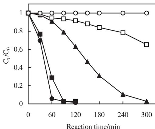
Fig. 8. Substituent effect on the nitration of PYH by NO<sub>2</sub>. ●: 1-MeOPY, ■: 1-MePY, ▲: PYH, □: 1-BrPY, ○: 1-NO<sub>2</sub>PY, [PYH] = 1.24 mmol dm<sup>-3</sup>, [NO<sub>2</sub>] = 100 ppm.
