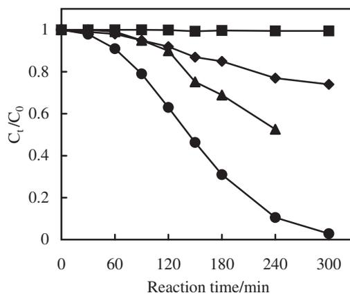
Fig. 7. Solvent effect on the nitration of PYH by NO<sub>2</sub>. ●: CH<sub>3</sub>CN, ▲: CH<sub>3</sub>OH, ◆: CH<sub>2</sub>Cl<sub>2</sub>, ■: CHCl<sub>3</sub>, [PYH] = 1.24 mmol dm<sup>-3</sup>, [NO<sub>2</sub>] = 100 ppm.
