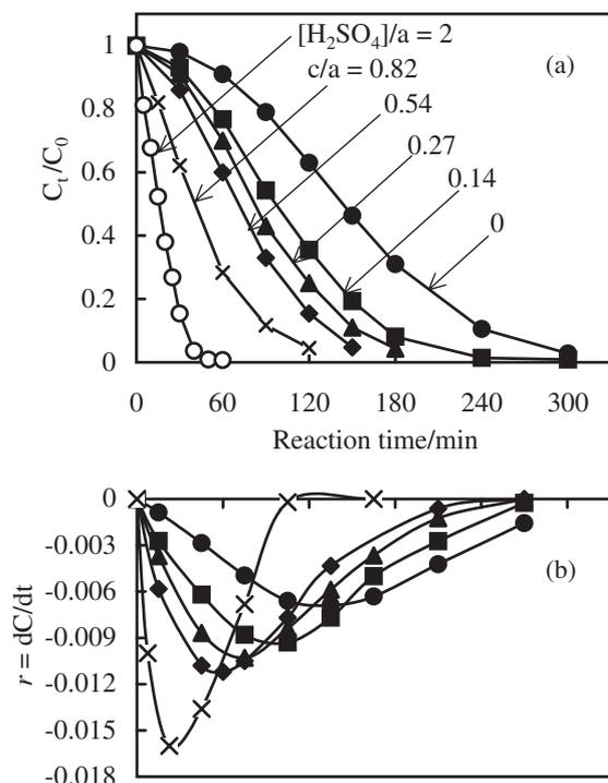
Fig. 5. Effect of previous aeration time of HNO<sub>3</sub> gas and addition of H<sub>2</sub>SO<sub>4</sub> in place of HNO<sub>3</sub> gas on the decay of PYH by NO<sub>2</sub>. ●: 0 min, ■: 20 min, ▲: 40 min, ◆: 80 min, ×: 120 min, ○: H<sub>2</sub>SO<sub>4</sub> (2.48 mmol dm<sup>-3</sup>), [PYH] = 1.24 mmol dm<sup>-3</sup>, [NO<sub>2</sub>] = 100 ppm, [HNO<sub>3</sub>] = 10.3 ppm.
