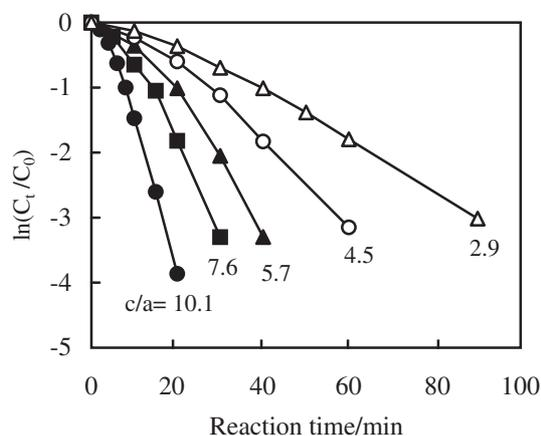
Fig. 10. Plot of  $\ln(C_t/C_0)$  versus time for the nitration of PYH by NO<sub>2</sub> in the presence of excess HNO<sub>3</sub>. [PYH] = 1.24 mmol dm<sup>-3</sup>, [NO<sub>2</sub>] = 100 ppm, [HNO<sub>3</sub>] = 3.6–12.5 mmol dm<sup>-3</sup>.
