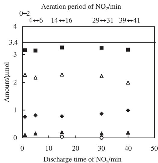
Fig. 1. Conversion products of NO<sub>2</sub> in acetonitrile and their material balance.  $\Delta$ : HNO<sub>3</sub> + HNO<sub>2</sub>,  $\blacklozenge$ : NO<sub>2</sub>(Insoluble),  $\blacktriangle$ : NO(Insoluble),  $\circ$ : NO<sub>2</sub> + NO(Soluble),  $\blacksquare$ : Total, [NO<sub>2</sub>] = 100 ppm.
