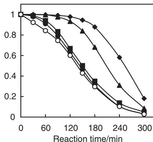
Fig. 14. Effect of previous aeration time of  $\text{HNO}_2$  gas and addition of urea on the decay of PYH by  $\text{NO}_2$ . ●: 0 min, ■: 20 min, ▲: 80 min, ◆: 120 min, ○:  $[\text{urea}] = 2.48$  mmol dm<sup>-3</sup>,  $[\text{PYH}] = 1.24$  mmol dm<sup>-3</sup>,  $[\text{NO}_2] = 100$  ppm,  $[\text{HNO}_2] = 11.1$  ppm.
