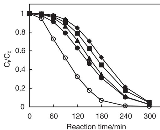
Fig. 6. Addition effect of water to acetonitrile on the nitration of PYH by NO<sub>2</sub>. Water content/ppm: ◆: 4200, ■: 3000, ▲: 1500, ●: 447, ○: 180, [PYH] = 1.24 mmol dm<sup>-3</sup>, [NO<sub>2</sub>] = 100 ppm.
