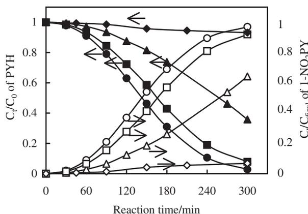
Fig. 3. Effect of  $\text{NO}_2$  concentration on the decay of PYH and on the increase in 1- $\text{NO}_2\text{PY}$  with time.  $[\text{PYH}] = 1.24 \text{ mmol dm}^{-3}$ ,  $[\text{NO}_2]/\text{ppm}$ :  $\blacklozenge, \blacktriangle, \blacksquare, \bullet$ : 10,  $\blacktriangle, \triangle, \blacksquare, \bullet$ : 50,  $\blacksquare, \bullet, \circ$ : 75,  $\bullet, \circ$ : 100, PYH: Black, 1- $\text{NO}_2\text{PY}$ : White.
