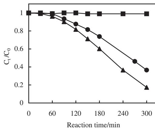
Fig. 4. Effect of added  $\text{HNO}_3$  gas on the decay of PYH by  $\text{NO}_2$ .  $[\text{PYH}] = 1.24 \text{ mmol dm}^{-3}$ ,  $\blacksquare$ :  $\text{HNO}_3$  (49 ppm),  $\bullet$ :  $\text{NO}_2$  (50 ppm),  $\blacktriangle$ :  $\text{NO}_2$  (50 ppm) +  $\text{HNO}_3$  (5 ppm).
