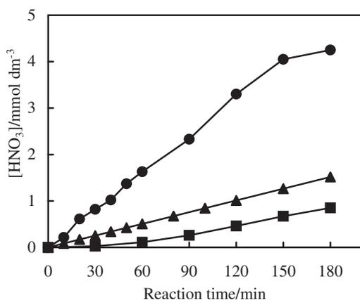
Fig. 9. Time course of the concentration of HNO<sub>3</sub> formed by Paths A, B, and C. ●: Path A, ■: Path B, ▲: Path C, Path A: [NO<sub>2</sub>] = 100 ppm, Path B: [PYH] = 1.24 mmol dm<sup>-3</sup>, [NO<sub>2</sub>] = 100 ppm, Path C: [HNO<sub>3</sub>] = 10.3 ppm.
