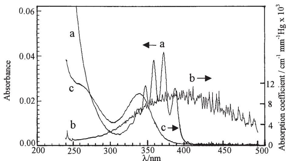
Fig. 12. UV-vis spectra of the nitrogenous species (curve a) formed by aerating NO<sub>2</sub> in acetonitrile together with those of NO<sub>2</sub> (curve b) and N<sub>2</sub>O<sub>4</sub> (curve c). [NO<sub>2</sub>] = 100 ppm, aeration time = 60 min.
