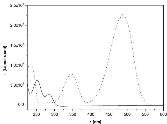
Figure 4. UV/visible spectrum of NBDPZ (dotted) compared to that of 1-(2-methoxyphenyl)piperazine (MPP, solid). Solvent, acetonitrile;  $C_{\text{NBDPZ}} = 1.1 \times 10^{-4}$  mol/L;  $C_{\text{MPP}} = 1.1 \times 10^{-4}$  mol/L.
