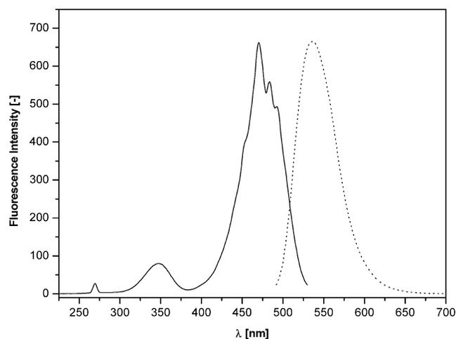
Figure 2. Fluorescence spectrum of methyl isocyanate NBDPZ (MI-NBDPZ) in acetonitrile/dimethyl sulfoxide 20:1 (v/v).  $C_{\text{MI-NBDPZ}} = 1.3 \times 10^{-5}$  mol/L;  $\lambda_{\text{exc}} = 470$  nm;  $\lambda_{\text{em}} = 537$  nm.
