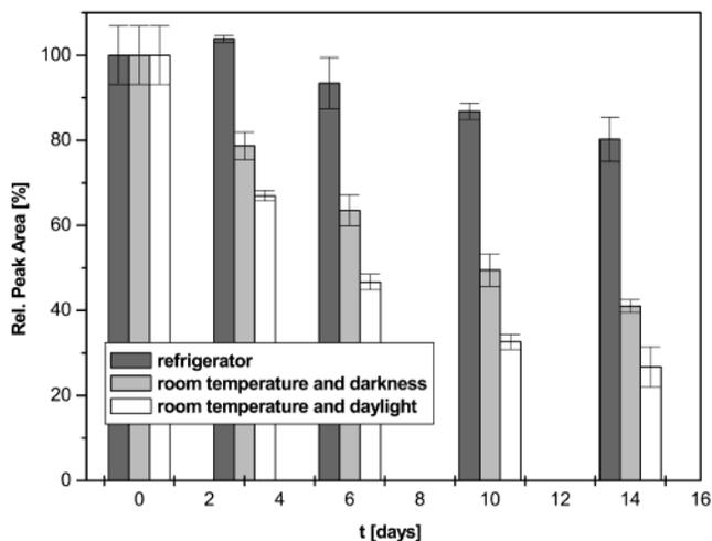
Figure 6. Stability of NBDPZ dissolved in acetonitrile applying three different storage conditions.  $c_{\text{NBDPZ}} = 5.5 \times 10^{-6} \text{ mol/L}$ ; HPLC analysis was performed using column 1 and gradient A; detection wavelength was 478 nm.
