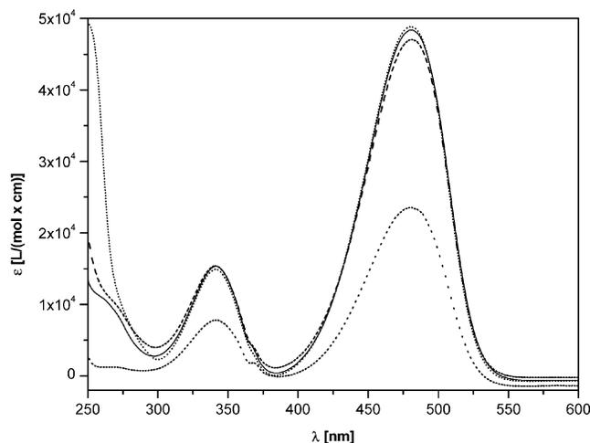
Figure 1. UV/visible spectra of selected NBDPZ isocyanate derivatives dissolved in acetonitrile/dimethyl sulfoxide 20:1 (v/v): methyl isocyanate (dotted), 2,6-toluene diisocyanate (dashed), methylene bis(phenyl isocyanate) (short dotted), and isophorone diisocyanate (solid). Concentrations range from  $1.2$  to  $1.6 \times 10^{-5}$  mol/L.
