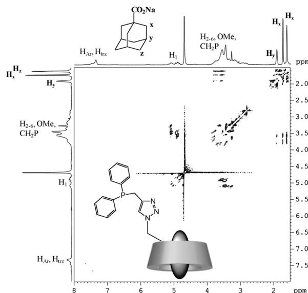
**Fig. 3** 2D TROESY NMR spectrum of a 1:1 mixture of AdCO<sub>2</sub>Na/1 in  $D_2O$  (25 °C, 6 mM/2 mM) and schematic representation of this inclusion complex.
