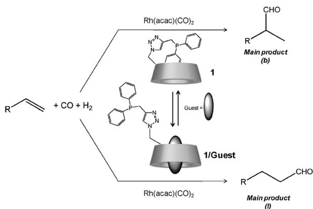
**Scheme 2** Schematic representation of the mechanism leading to linear or branched products.
