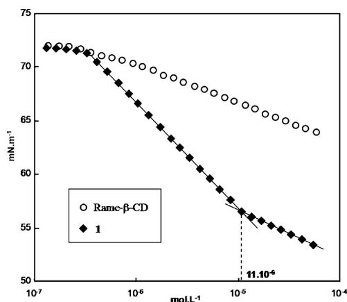
**Fig. 2** Surface tension curve of aqueous solutions of **1** and Rame- $\beta$ -CD at 25 °C.
