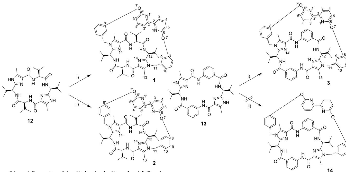
Scheme 4. Preparation of the chiral molecular hinges **1** and **2**. Reaction conditions: i) **8**, Cs<sub>2</sub>CO<sub>3</sub>, CH<sub>3</sub>CN,  $\Delta$ , 25%; ii) **11**, Cs<sub>2</sub>CO<sub>3</sub>, CH<sub>3</sub>CN,  $\Delta$ , 16%.
