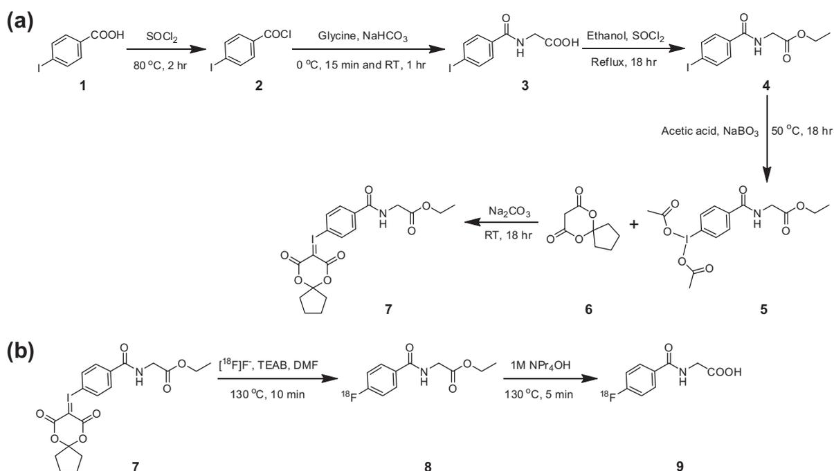
Figure 1. Synthesis of (a) iodonium ylide precursor and (b) [ $^{18}\text{F}$ ]PFH.
