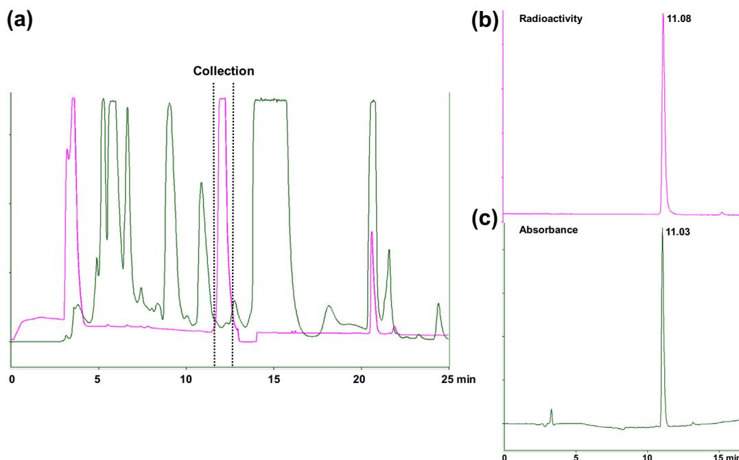
**Figure 2.** HPLC chromatograms of (a) [ $^{18}\text{F}$ ]PFH batch obtained while purification, (b) [ $^{18}\text{F}$ ]PFH obtained while quality control, and (c) non-radioactive PFH standard.
