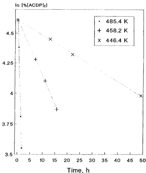
Figure 1. Representation through first-order kinetic plots of the data obtained in typical experiments of the gas-phase ACDP thermolysis in the presence of *n*-octane (unpacked reactors).
