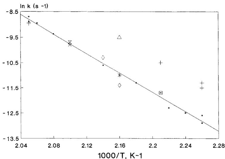
Figure 2. Arrhenius equation plot for the gas-phase ACDP thermolysis in the presence of *n*-octane, in the 443–488 K temperature range. Symbols: (□) unpacked vessels; (+) packed vessels; (\*) toluene added (ca. 8 torr); (◇) 1,4-cyclohexadiene added (ca. 9 torr); (×) acetone added (ca. 13 torr); (⊠) Di-*tert*-butyl peroxide added (ca. 5 torr); (Δ) 1,4-cyclohexadiene added, packed reactors (ca. 40 torr); and (□) reactor previously silanized.
