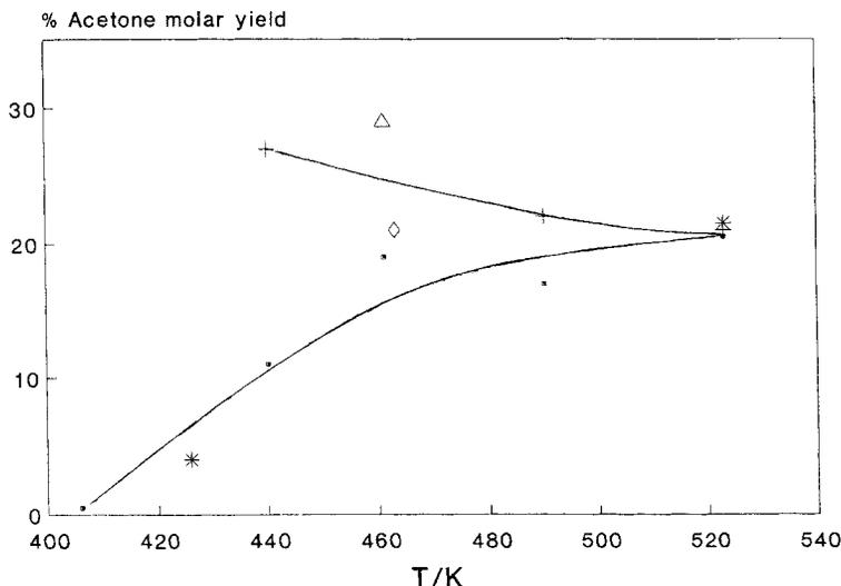
Figure 3. Temperature effect on the acetone molar yields of the gas-phase ACDP thermolysis in the presence of *n*-octane. Symbols: (□) unpacked vessel; (+) packed vessel; (\*) toluene added (ca. 6 torr); (◇) 1,4-cyclohexadiene added (ca. 9 torr); and (△) 1,4-cyclohexadiene added, packed reactor (ca. 40 torr).
