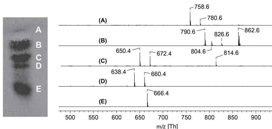
**Fig. 3.** Left: image of a typical HPTLC plate used to separate the oxidation products of PLPC after incubation with the Fenton reagents (cf. Section 2) for 16 h. Staining was performed by using the non-destructive dye primuline. Right: positive ion MALDI-TOF mass spectra recorded to confirm the identities of the lipids detectable in the individual TLC fractions. Peak assignments are available in Table 1.
