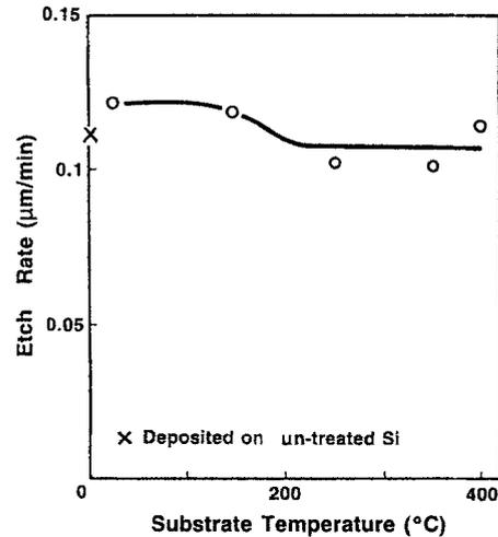
Fig. 5. Dependence of etch rate of deposited films on temperature of 1 min plasma treatment in  $N_2$ , when deposited at 400°C with 4.2% ozone.
