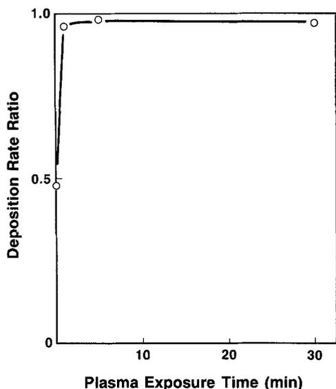
Fig. 1. Dependence of NSG deposition rate ratio on plasma exposure time, when plasma-treated at 350°C in N<sub>2</sub> deposited at 400°C with 4.2% ozone.
