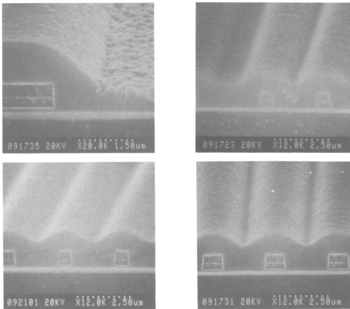
Fig. 3. Surface morphology and step coverage of films plasma-treated at 350°C in N<sub>2</sub> for 0 min (a, top left), 1 min (b, top right), 10 min (c, bottom left), and 30 min (d, bottom right), and deposited on polysilicon lines on thermal oxide at 400°C with 5% ozone.
