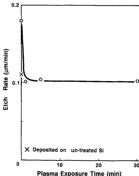
Fig. 2. Dependence of etch rate of films deposited at 400°C with 4.2% ozone on time of plasma treatment made at 350°C in N<sub>2</sub>.
