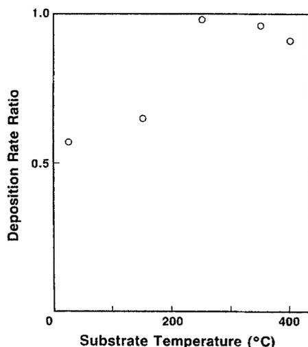
Fig. 4. Dependence of deposition rate ratio on temperature of 1 min plasma treatment in  $N_2$ , when deposited at 400°C with 4.2% ozone.
