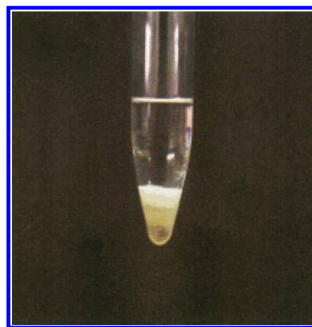
Figure 4. Separated phases after centrifugation of the reaction mixture of the aldol reaction of benzaldehyde with 2 in the presence of 1a . Upper phase: water, middle phase: 1a , lower phase: mixture of organic compounds.
