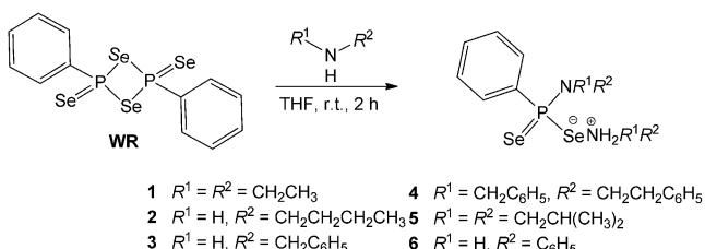
**Scheme 1.** Synthesis of ammonium phenylphosphonamidodiselenoates **1–6**.
