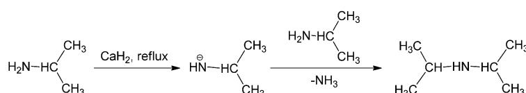
**Scheme 3.** Formation of small amount of diisopropylamine (ca. 5 % based on  $^1\text{H}$  NMR spectroscopic analysis) in isopropylamine purification process.
