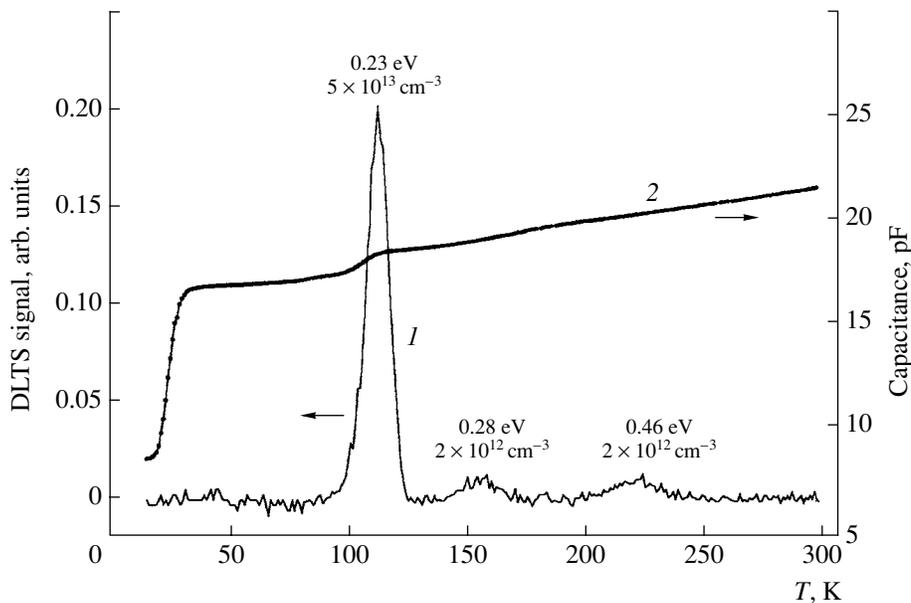
**Fig. 3.** (1) DLTS spectrum and (2) temperature-dependent capacitance of the Schottky contact for silicon epilayers grown from the first silane batch; the numbers at the peaks specify the concentrations and ionization energies of the corresponding levels; the carrier concentration in the epilayers at  $T = 300 \text{ K}$ ,  $V_{\text{sample}} = 4 \text{ V}$ , and  $f = 400 \text{ kHz}$  is  $n = 4 \times 10^{14} \text{ cm}^{-3}$ .
