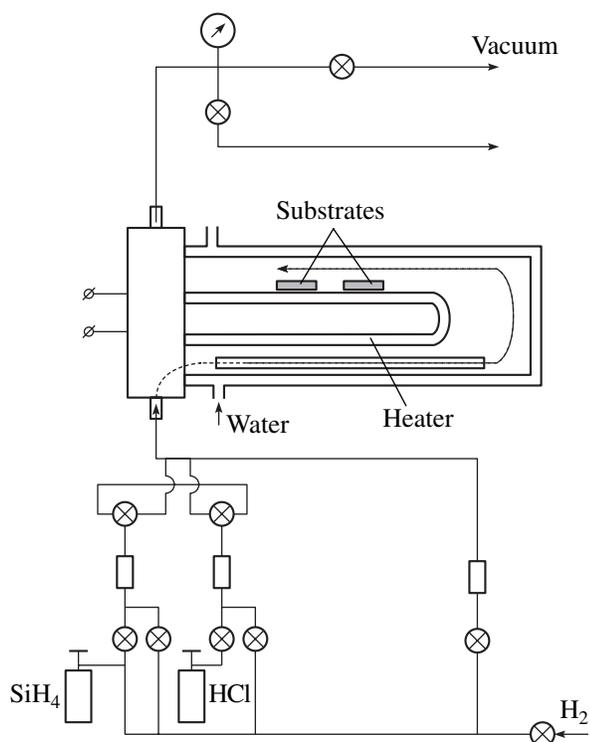
**Fig. 1.** Schematic of the apparatus for the growth of silicon epilayers.
