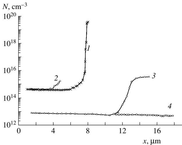
**Fig. 2.** Impurity profiles in silicon epilayers grown using two batches of silane: (1, 2) first purification (simple distillation), (3, 4) second purification (fractional distillation); measurements on (1, 3) electrolyte/silicon and (2, 4) Au/Si contacts.
