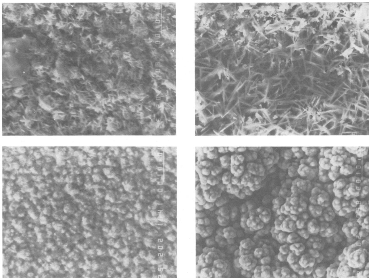
Fig. 9. Influence of pulse length ( $t_{on}$ ) on the morphology of the deposit of the Pb/Sn alloy with pulse current density ( $I_p$ ) = 34.44 A/dm<sup>2</sup> and period ( $T = t_{on} + t_{off}$ ) = 50 ms. The values of  $t_{on}$  (ms) are (a, top left) 0.2; (b, top right) 0.5; (c, bottom left) 1.0; (d, bottom right) 2.0.
