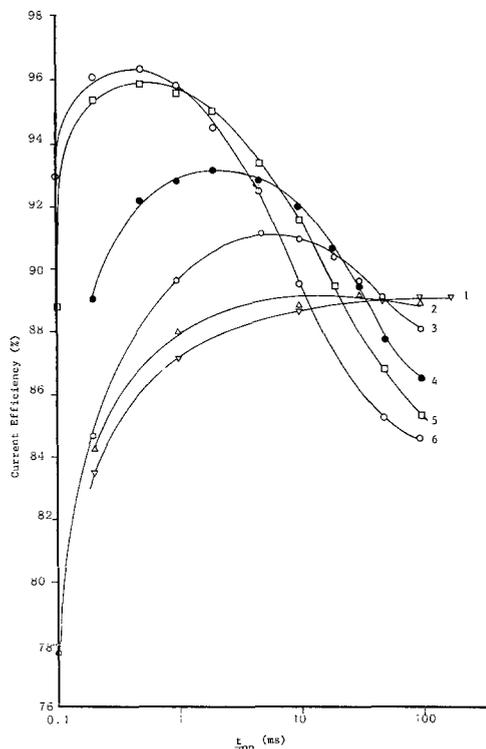
Fig. 1. Influence of pulse length ( $t_{on}$ ) on current efficiency of Pb/Sn deposition at different pulse current density ( $I_p$ ) with duty cycle = 25%. The pulse current densities are: curve 1:0.54, curve 2:2.15, curve 3:4.31, curve 4:8.61, curve 5:17.22, curve 6:34.44 A/dm<sup>2</sup>.
