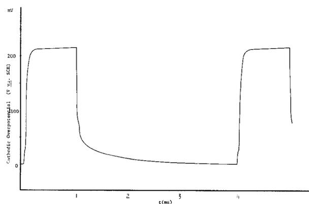
Fig. 8. The cathodic overpotential diagram under the pulse current with I<sub>p</sub> = 16.22, t<sub>on</sub> = 1 ms, and duty cycle = 25%.
