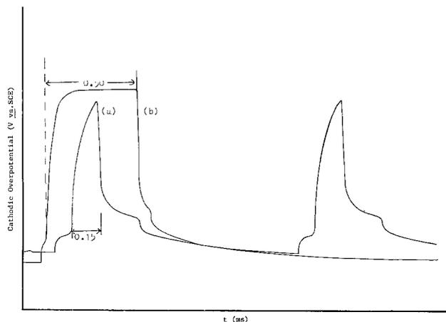
Fig. 6. The cathodic overpotential diagram of Pb/Sn system at different pulse length (t<sub>on</sub>) with pulse current density (I<sub>p</sub>) = 17.22 A/dm<sup>2</sup> and duty cycle = 25%. The values of t<sub>on</sub> (ms) are: (a) 0.15, (b) 0.50.
