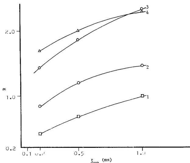
Fig. 10. Predomination of the lead in the lead-tin alloy as a function of the on-time with pulse current density ( $I_p$ ) = 34.44 A/dm<sup>2</sup> and duty cycle = 25%.
