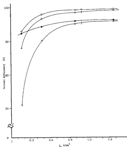
Fig. 4. Influence of pulse current density ( $I_p$ ) on current efficiency at different plating systems with pulse length ( $t_{\text{on}}$ ) = 50 ms and duty cycle = 25%. The systems are curve 1, Pb/Sn; curve 2, Pb; curve 3, Sn; curve 4, Cu ( $\text{H}_2\text{SO}_4$ ).
