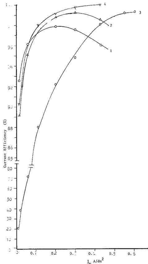
Fig. 3. Influence of current density on current efficiency at different plating systems with the direct current. The systems are curve 1, Pb/Sn; curve 2, Pb; curve 3, Sn; curve 4, Cu ( $\text{H}_2\text{SO}_4$ ).
