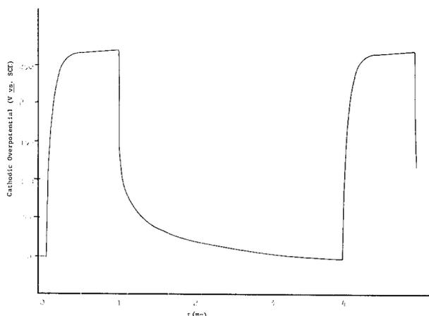
Fig. 7. The cathodic overpotential diagram under the pulse current with I<sub>p</sub> = 8.61, t<sub>on</sub> = 1 ms, and duty cycle = 25%.
