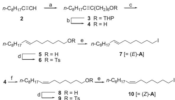
**Scheme 2.** Synthesis of the building blocks (*E*)-**A** (= **7**) and (*Z*)-**A** (= **10**). Reagents: (a) *n*-BuLi, I(CH<sub>2</sub>)<sub>6</sub>OTHP, THF, HMPA; (b) *p*-TsOH, MeOH (82%, two steps); (c) LiAlH<sub>4</sub>, THF, diglyme (97%); (d) *p*-TsCl, C<sub>5</sub>H<sub>5</sub>N (96% for **6**; 87% for **9**); (e) NaI, DMF (89% for **7**; 97% for **10**); (f) H<sub>2</sub>, Lindlar's Pd cat., quinoline, cyclohexane (99%).
