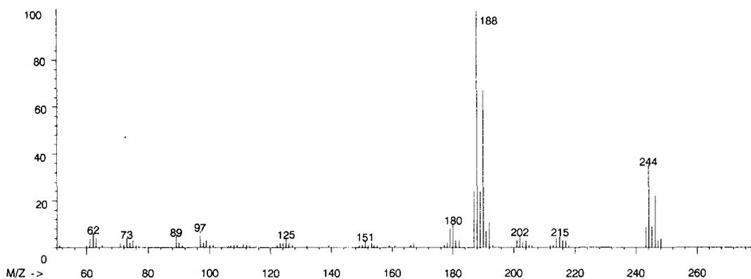
**Fig.3** Mass spectral data of butyl-boronic acid ester of 3,6-dichlorocatechol
