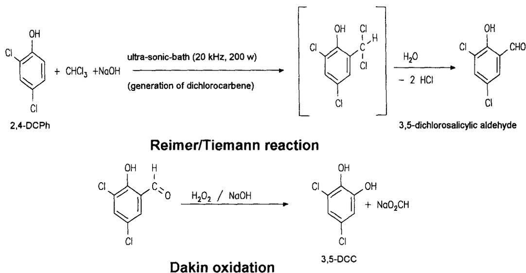
**Fig.4** Reaction scheme of Reimer/Tiemann reaction of 2,4-Dichlorophenol and subsequent Dakin oxidation leading to 3,5-Dichlorocatechol.
