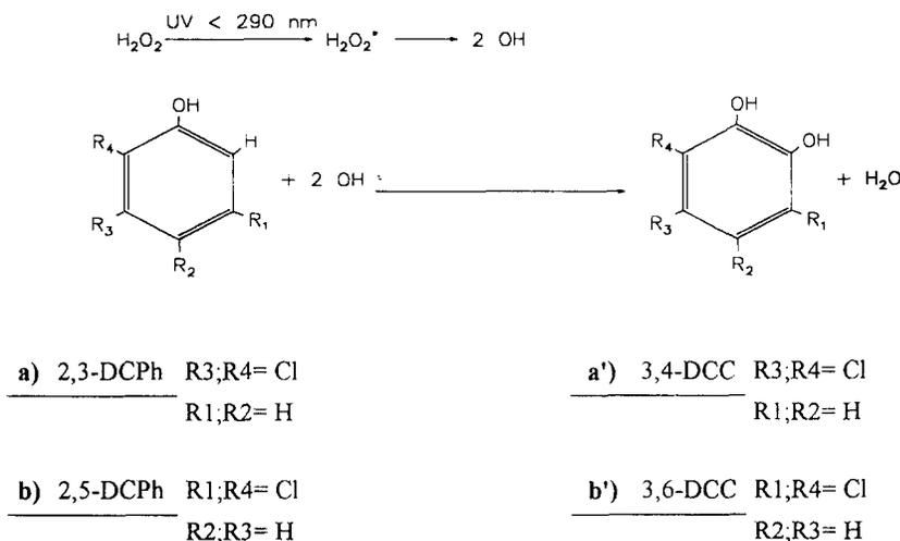
**Fig.1** Reaction scheme of UV-photoradical synthesis of 3,4- and 3,6-DCC
