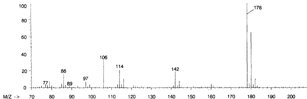
**Fig.2** Mass spectrum of 3,6-DCC obtained after flow-injection of an methanolic solution into a particle-beam-interface/MS.
