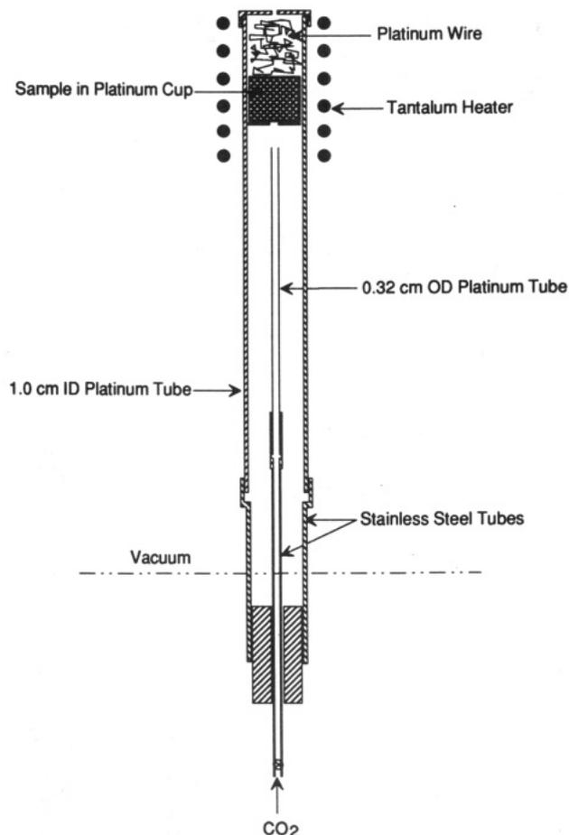
Figure 1. Schematic diagram of the platinum Kudsen cell arrangement.
