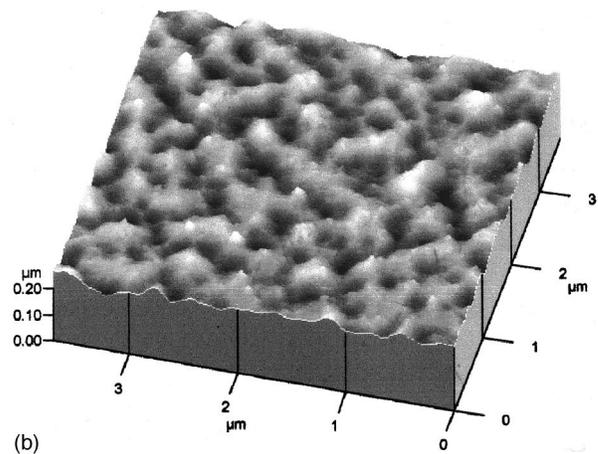
FIG. 3. The AFM image of interface between poly-Si and  $\text{Li}^2\text{Ox}$  fabricated by new method. (a) Laser energy density is  $283 \text{ mJ/cm}^2$ . The rms surface roughness of the interface is  $23 \text{ \AA}$ . (b) The AFM image of surface morphology of poly-Si recrystallized from *a*-Si by conventional method. Laser energy density is  $283 \text{ mJ/cm}^2$ . The rms surface roughness of poly-Si is  $111 \text{ \AA}$ .
