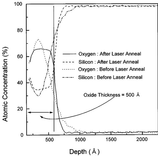
FIG. 1. The oxygen and silicon atomic concentration analyzed by AES before and after excimer laser irradiation.
