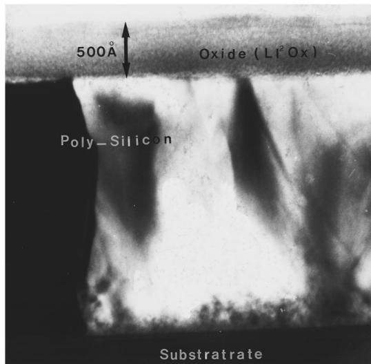
FIG. 2. TEM image of fabricated  $\text{Li}^2\text{Ox}$  and poly-Si. The scale of the image is 1:250000. The sample was irradiated with laser energy density of  $371 \text{ mJ/cm}^2$ . The  $\text{Li}^2\text{Ox}$ , fully recrystallized poly-Si, and clean interface of  $\text{Li}^2\text{Ox}$  and poly-Si is observed.
