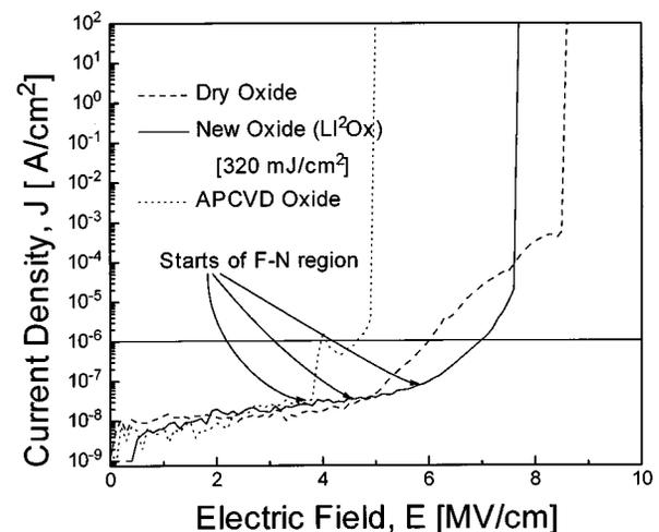
FIG. 4. The oxide breakdown electric field in  $\text{Li}^2\text{Ox}$ , APCVD oxide, and thermal dry oxide grown from poly-Si.
