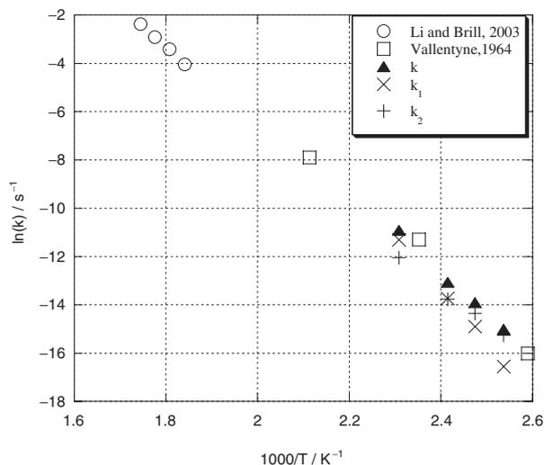
**Figure 2.** The Arrhenius diagram for the apparent decrease rate constants  $k$  of threonine together with the literature data.<sup>5,10</sup>
