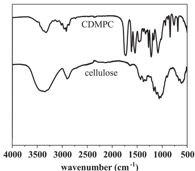
**FIGURE 3** Fourier-transform infrared (FT-IR) spectra of cellulose and CDMPC
