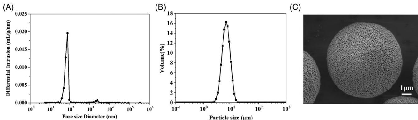
**FIGURE 2** (A) pore size distribution, (B) particle size distribution, and (C) SEM image of the wide pore silica
