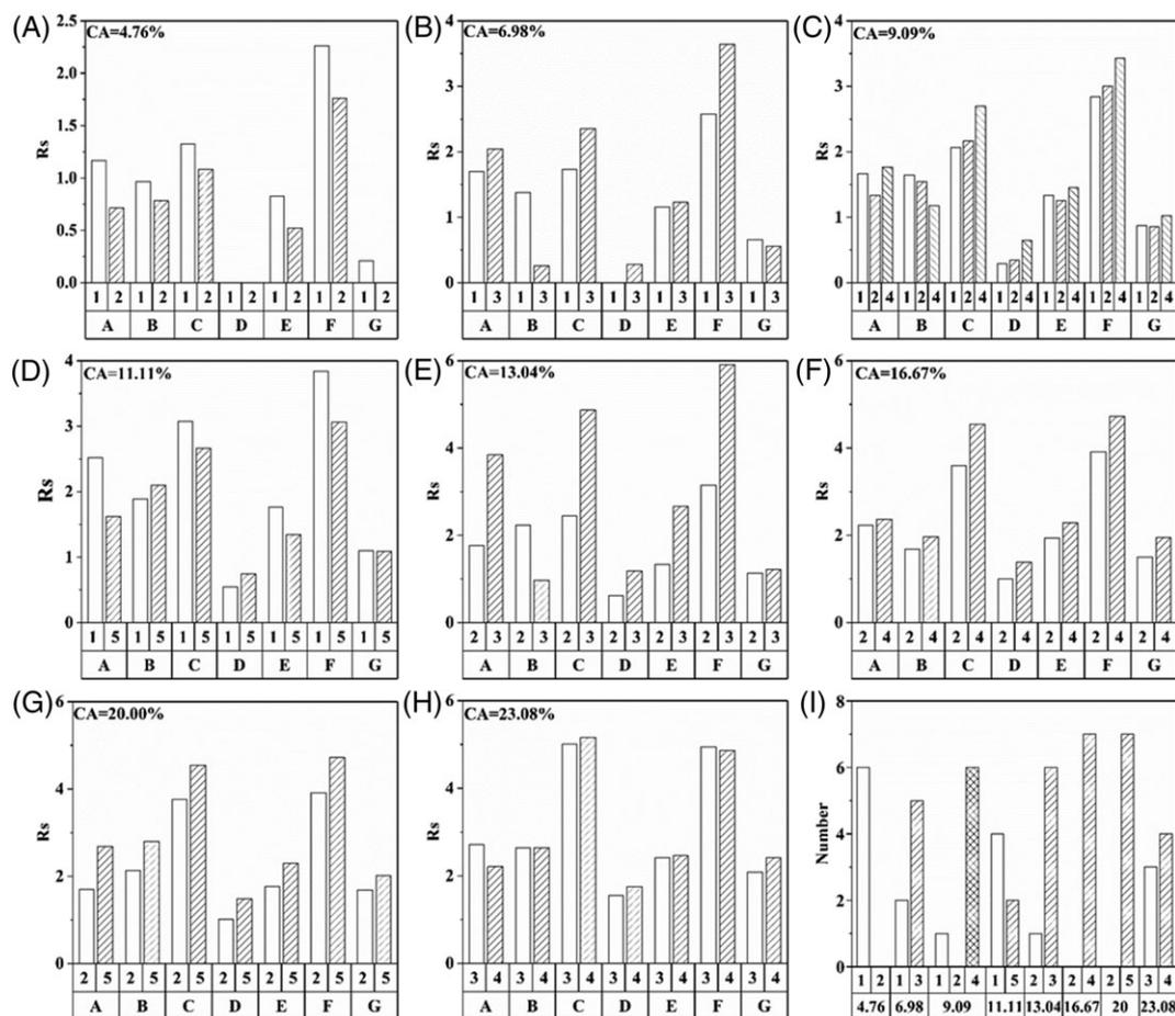
**FIGURE 7** Resolution of seven racemates on chiral stationary phases (CSPs) in eight groups (A-H), and the racemates number of achieving better resolution on the two or three CSPs in each group (I). CA is the coating amount. The first line of the abscissa in each figure represents the coating times, and the second line represents the racemates to be separated (A-H) or the total coating amount (I)
