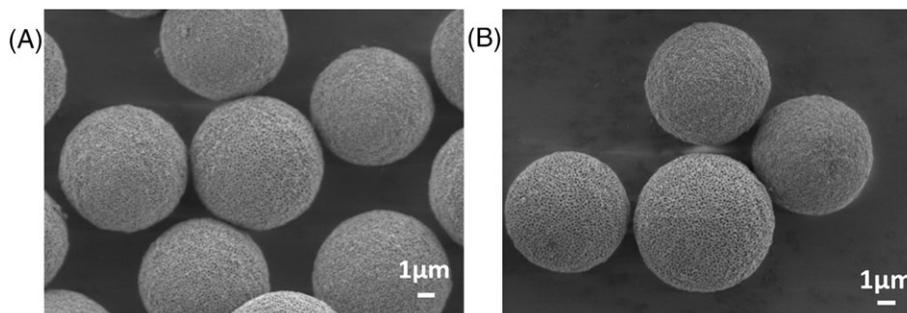
**FIGURE 6** SEM image of (A) uncoated silica and (B) CSP-0.20-3
