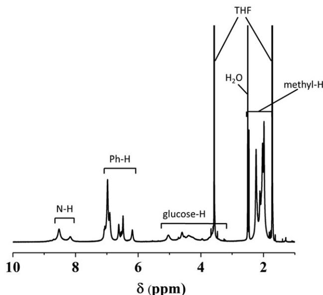
**FIGURE 4**  $^1\text{H}$  NMR spectrum of CDMPC in tetrahydrofuran- $d_8$  (700 MHz)
