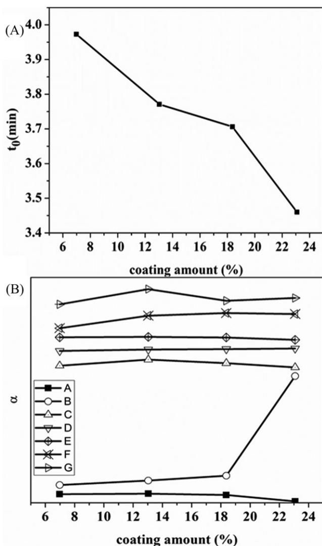
**FIGURE 11** The influence of coating amount on dead time (A) and separation factor (B)
