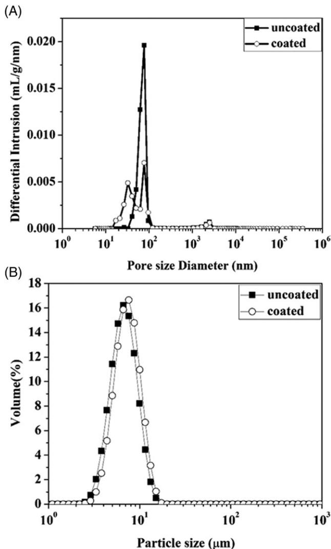
**FIGURE 5** The pore size distribution (A) and particle distribution (B) of uncoated silica and the CSP-0.15-4
