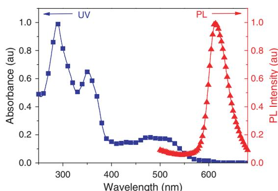
**Fig. 2.** UV-visible absorption and PL spectra of  $(\text{tq})_2\text{Ir(III)(acac)}$  in  $\text{CH}_2\text{Cl}_2$ .
