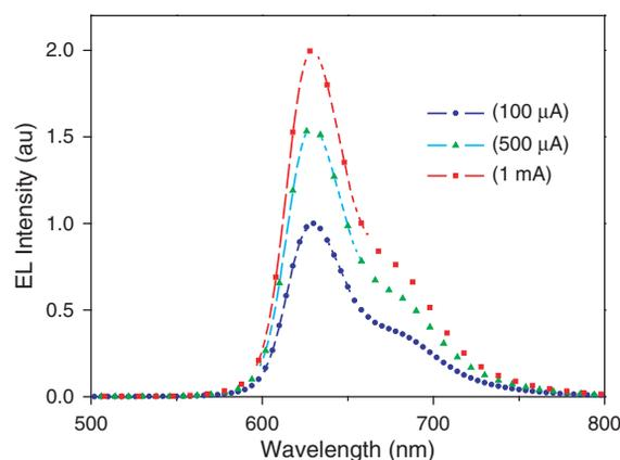
**Fig. 4.** EL spectra of the fabricated devices at different currents.
