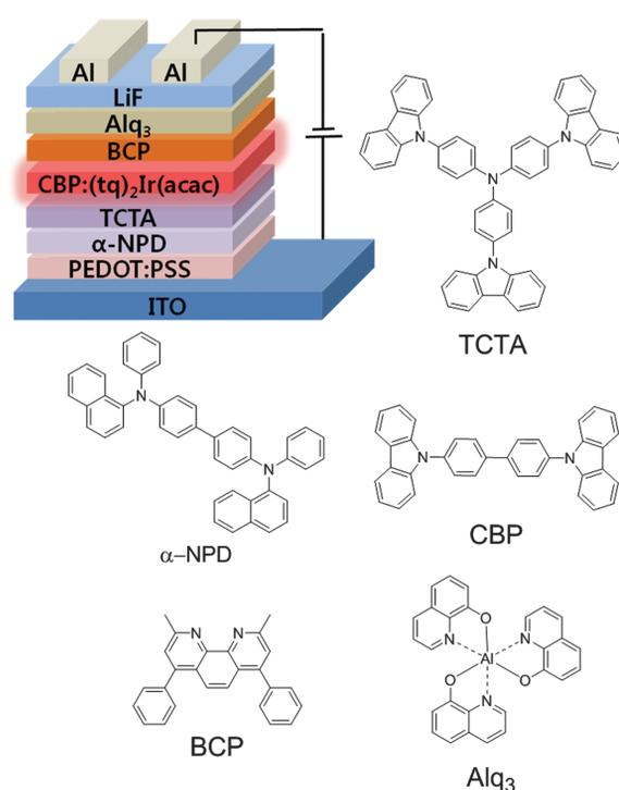
**Fig. 3.** The fabricated EL device structure and the materials used for each layer of the device.
