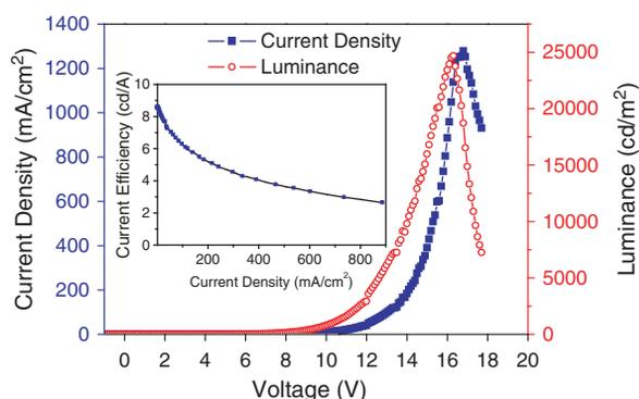
**Fig. 5.**  $I$ - $V$ - $L$  characteristics of the device and current efficiency versus current density of the device (inset).
