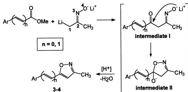
Fig. 2. General method for synthesis of isoxazole derivatives **3–4** from carboxylic esters.
