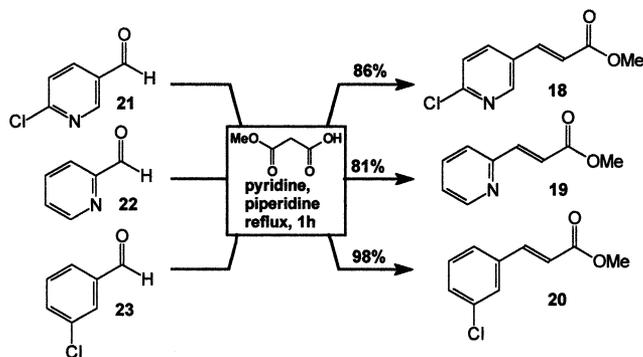
Fig. 4. Synthesis of  $\alpha,\beta$ -unsaturated aromatic or heteroaromatic methyl esters **18–20**.
