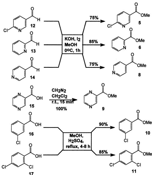
Fig. 3. Synthesis of aromatic or heteroaromatic methyl esters **5–6**, **8–11** from the corresponding aldehydes or carboxylic acid derivatives.
