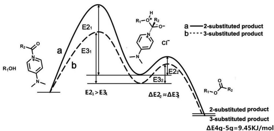
Figure 1. Proposed energy diagram for the DMAP-catalyzed esterification.
