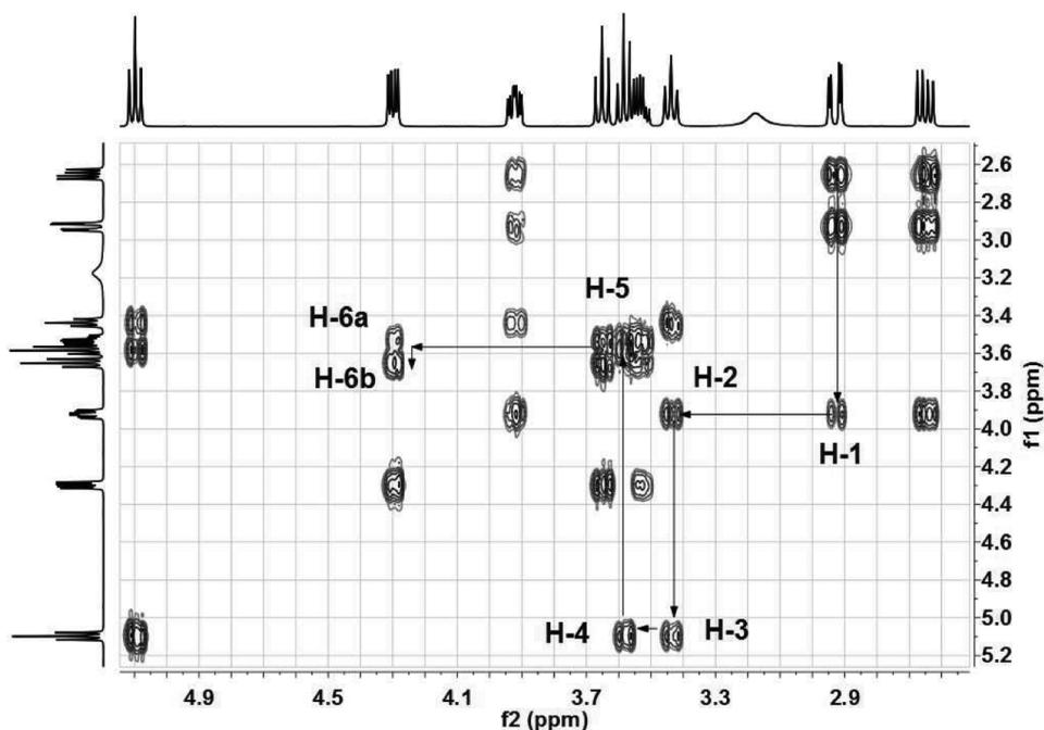
Figure 4.  $^1\text{H}$ - $^1\text{H}$  COSY spectra of **5a**.
