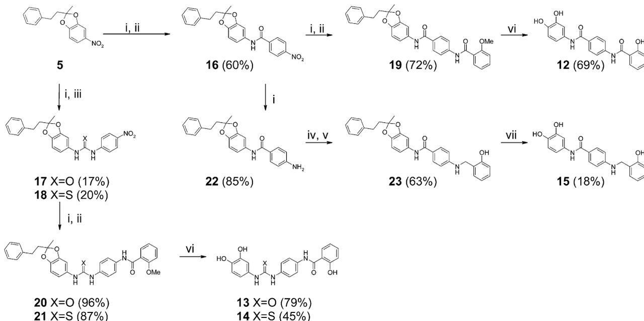
**Scheme 2.** Reagents and conditions: (i) 10% Pd-C/THF/H<sub>2</sub>; (ii) ArCOCl/Et<sub>3</sub>N/DMF/argon; (iii) 4-NO<sub>2</sub>PhNCO or 4-NO<sub>2</sub>PhNCS; (iv) 2-OH-PhCHO/THF/4Å molecular sieves/reflux; (v) Me<sub>4</sub>NBH(OAc)<sub>3</sub>/THF/reflux; (vi) BBr<sub>3</sub>/CH<sub>2</sub>Cl<sub>2</sub>/reflux; (vii) concd HCl (aq)/THF/reflux.
