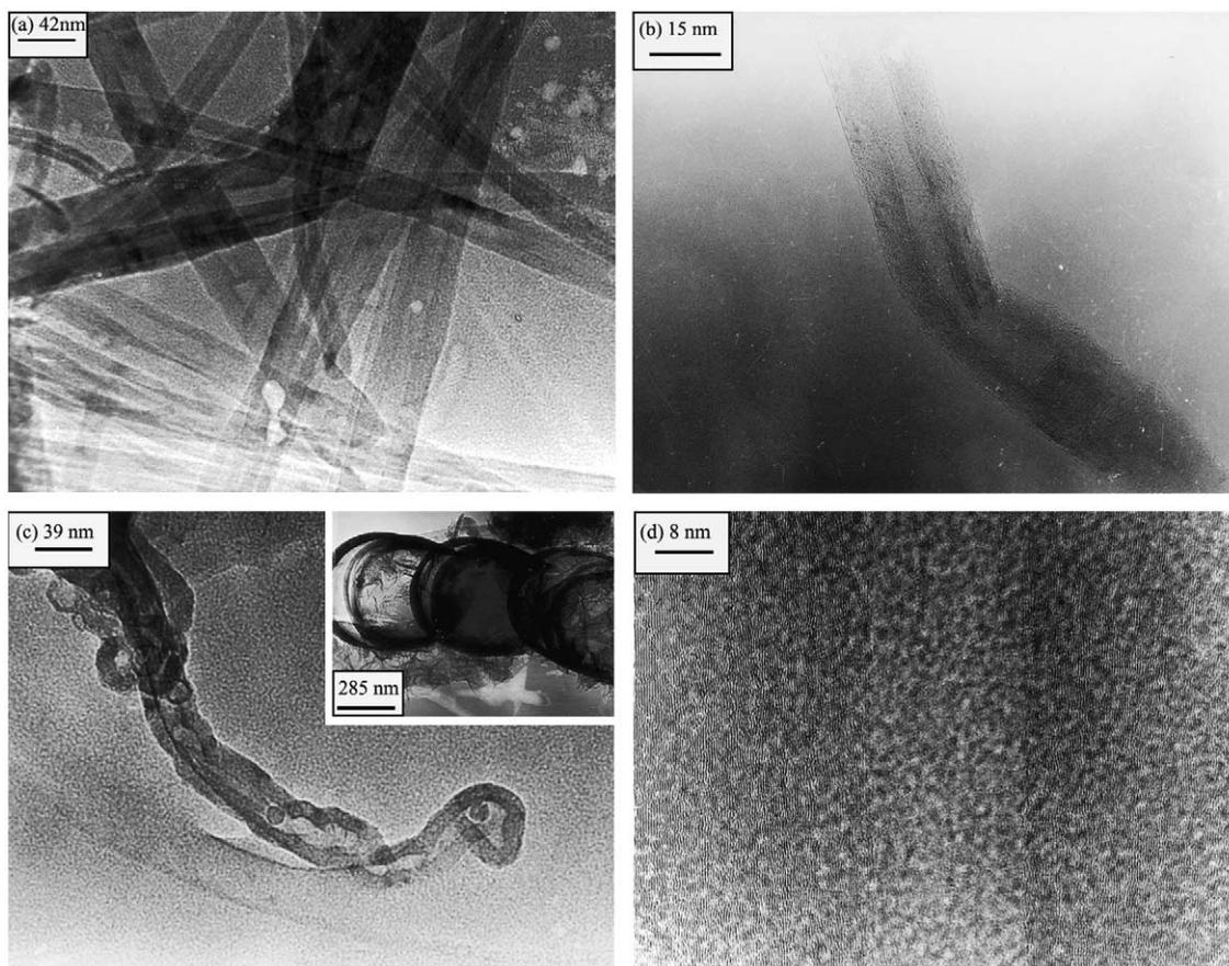
Fig. 3. TEM images of BN nanotubes obtained by procedure (ii): (a) a collection nanotube; (b) a nanotube with an interesting bend or kink; (c) nanotube showing an unusual cap; (d) a high-resolution image indicating the discontinuous lattice planes. Inset in (c) show bulbous structures found occasionally with the nanotubes.
