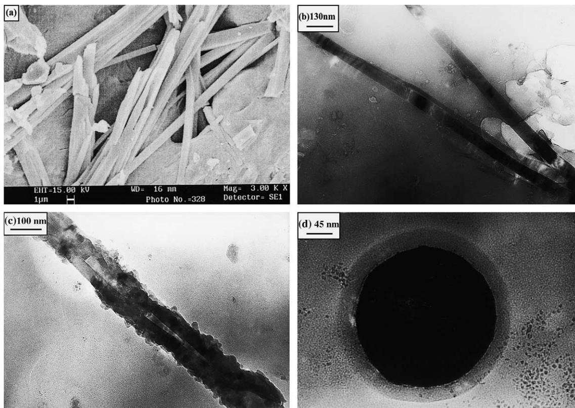
Fig. 4. Nanostructures of BN obtained by the reaction of  $H_3BO_3$  and catalytic Fe particles (dispersed over silica) with  $NH_3$  by procedure (iii): (a) SEM image of plates and whiskers; (b) TEM image of nanowires; (c) TEM image of a nanotube and (d) TEM image of a BN-coated Fe particle.
