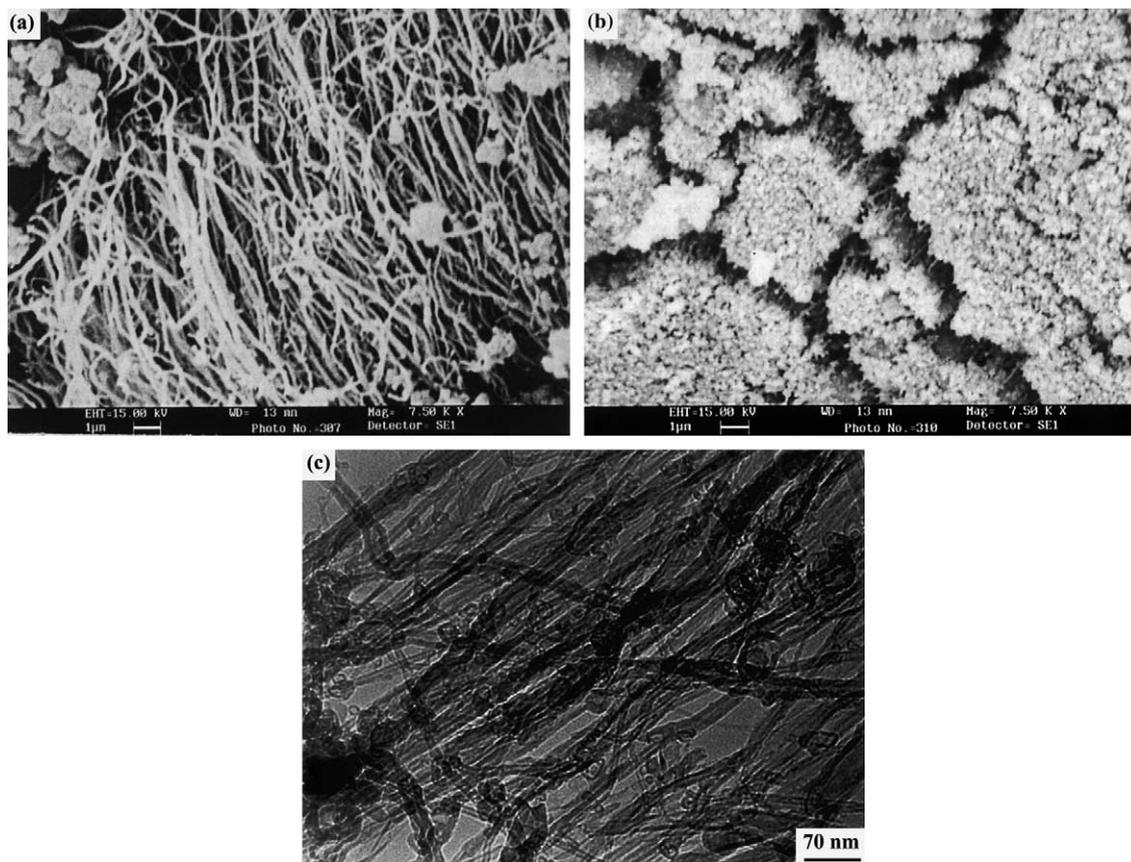
Fig. 2. SEM and TEM images of aligned BN nanotube bundles obtained by the reaction of  $\text{H}_3\text{BO}_3$  and aligned multi-walled carbon nanotubes with  $\text{NH}_3$  by procedure (ii): (a) and (b) give side and top view SEM images, respectively; (c) TEM image of pure BN nanotubes obtained at the mouth of the inner quartz tube.
