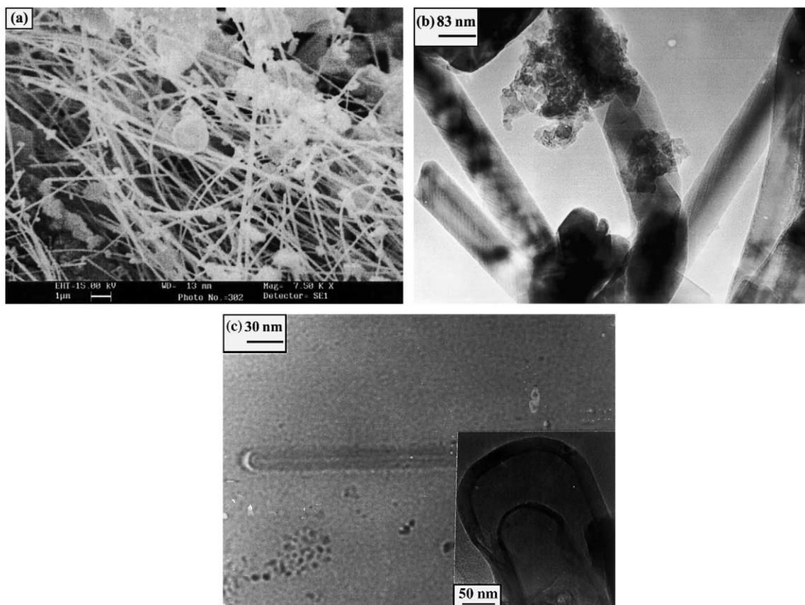
Fig. 1. Nanostructures obtained by the reaction of H<sub>3</sub>BO<sub>3</sub> and activated carbon with NH<sub>3</sub> by procedure (i): (a) SEM image; (b) TEM image of nanowires; (c) TEM image of a nanotube. Inset shows an interesting nanotube in a nanotube.
