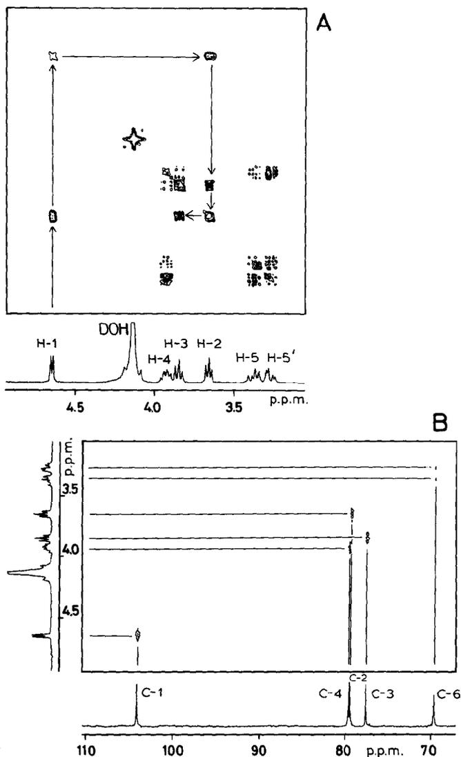
Fig. 3. Contour plot of 2D (A) H-H COSY and (B) C-H COSY spectra of stereoregular (1→5)- $\alpha$ -D-xylofuranan.
