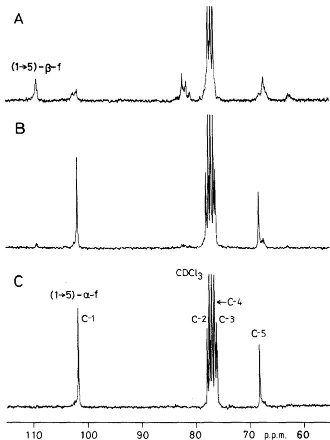
Fig. 1.  $^{13}\text{C}$ -N.m.r. spectra of (A) poly[1,5-anhydro-2,3-di-*O*-(*tert*-butyldimethylsilyl)- $\beta$ -D-xylofuranose] prepared by use of  $\text{SbCl}_5$  at  $-20^\circ$  and (B) prepared by use of  $\text{PF}_5$  at  $-60^\circ$ , and (C) 2,3-di-*O*-(*tert*-dimethylbutylsilyl)-(1 $\rightarrow$ 5)- $\alpha$ -D-xylofuranan.
