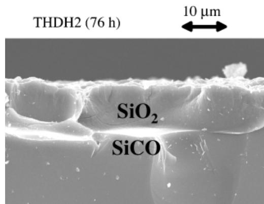
**Fig. 3.** Typical micrograph of the silica overlayer in the three samples with the lower carbon content.
