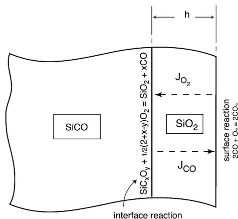
Fig. 2. The coupled diffusion problem in passive oxidation of an effluent system. The carbon monoxide evolved at the interface must diffuse out just as the oxygen diffuses toward the interface.
