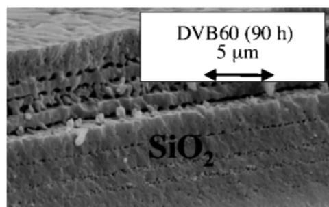
**Fig. 4.** Strings of bubbles, layered parallel to the interface in the sample with the highest carbon content.
