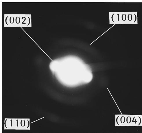
FIG. 4. Selected-area diffraction pattern of carbon nanotube inserted in Fig. 1(b).
