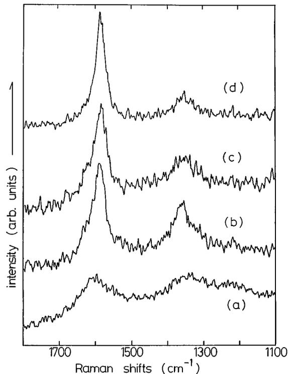
FIG. 2. Raman spectra of deposits obtained by CVD on heat-treated Ni films with initial thicknesses of (a) 1, (b) 5, (c) 10, and (d) 100 nm.
