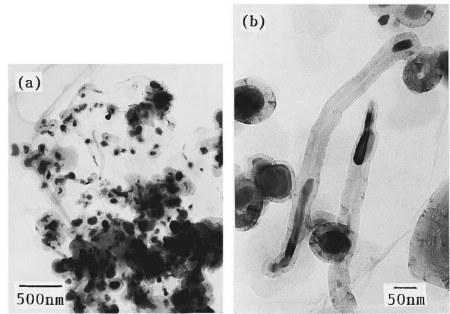
FIG. 5. Transmission electron micrographs of (a) carbon nanotubes and particles and (b) carbon tubes grown by CVD at 800 °C using a Ni thin film with thickness of 5 nm. The thick network is a microgrid made of organic material. Transparent carbon sheets are considered to be amorphous carbon.
