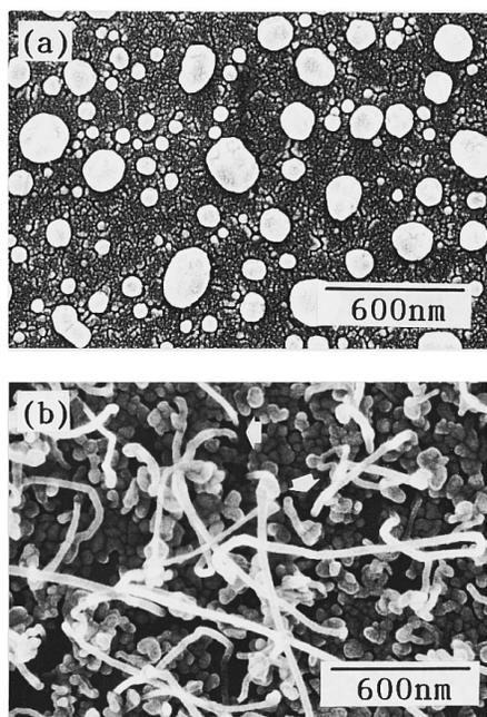
FIG. 1. Scanning electron micrographs of (a) heat-treated Ni film with thickness of 5 nm and (b) deposit obtained by CVD on Ni droplets appearing in (a). Temperature of heat treatment and CVD was 700 °C. Gold film with thickness about 10 nm was deposited for SEM observation.
