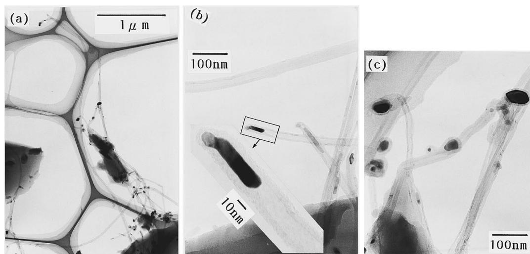
FIG. 3. Transmission electron micrographs of (a) carbon nanotubes and particles, (b) carbon nanotubes, and (c) carbon particles grown by CVD at 700 °C using Ni thin film with thickness of 5 nm. The thick network is a microgrid made of organic material. Large dark islands are broken pieces of quartz glass.
