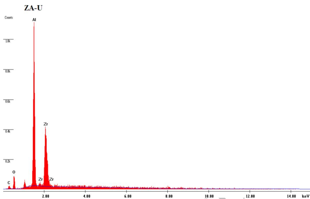
Figure 4c. EDAX spectrum of ZA-U solid acid catalyst.
