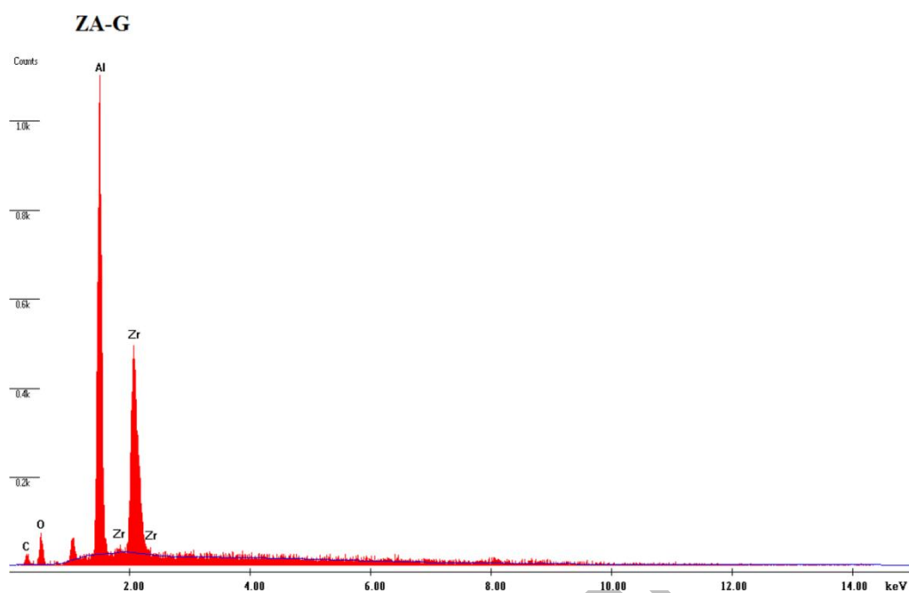
Figure 4e. EDAX spectrum of ZA-G solid acid catalyst.
