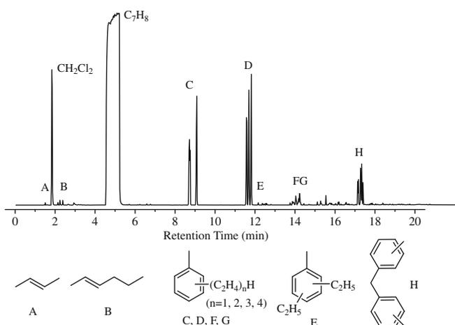
**Fig. 5.** GC-MS analysis of the products obtained from **2**/MAO in toluene at 0 °C.
