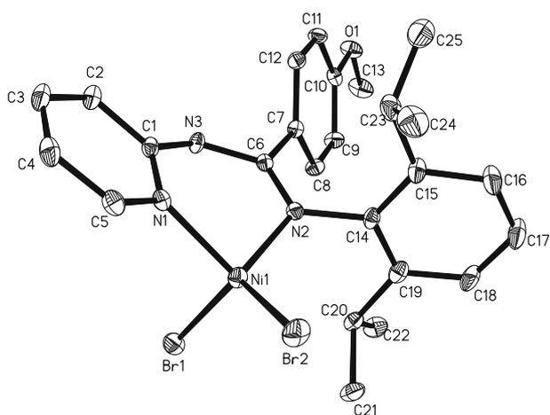
**Fig. 3.** Molecular structure of **3** depicted with 30% thermal ellipsoids and with hydrogen atoms omitted. Selected bond lengths (Å) and angles (°): C(1)–N(3) 1.397(4), C(6)–N(3) 1.370(4), C(6)–N(2) 1.298(4), C(14)–N(2) 1.453(5), Ni(1)–N(1) 1.984(3), Ni(1)–N(2) 1.968(3), Ni(1)–Br(1) 2.4006(7), Ni(1)–Br(2) 2.3342(7), N(1)–Ni(1)–N(2) 92.7(1), N(1)–Ni(1)–Br(1) 99.90(10), N(1)–Ni(1)–Br(2) 112.70(9), N(2)–Ni(1)–Br(1) 103.89(9), N(2)–Ni(1)–Br(2) 118.01(9), Br(1)–Ni(1)–Br(2) 123.94(3).
