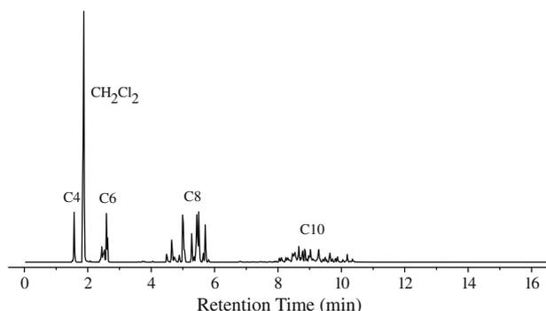
**Fig. 6.** GC-MS analysis of ethylene oligomers obtained by **2**/MAO in CH<sub>2</sub>Cl<sub>2</sub> at 0 °C (run 6 in Table 2).
