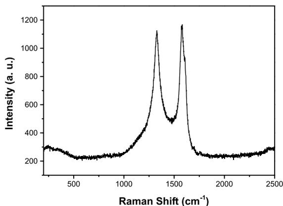
Fig. 2. Raman spectra of CNTs, showing multiwalled structure of CNTs.
