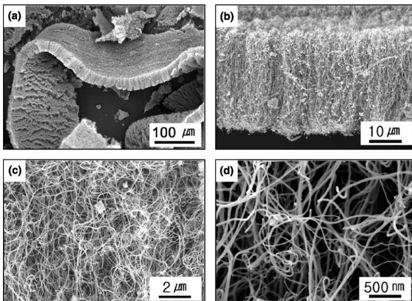
Fig. 1. SEM micrographs of deposits produced by W-based catalyst at 950 °C. (a) Large quantities of carpet-like deposits were scraped off the inner wall of the quartz tube. (b) Magnified view of (a), revealing that the deposits have a length about 30 μm. (c) Magnified view of (b). (d) High-resolution SEM image of deposits, showing the average diameter of about 20–40 nm.
