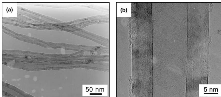
Fig. 3. (a) TEM image of CNTs, showing a multiwalled structure with a hollow inside. (b) HRTEM image of a CNT, showing high-crystallinity of graphite sheets.
