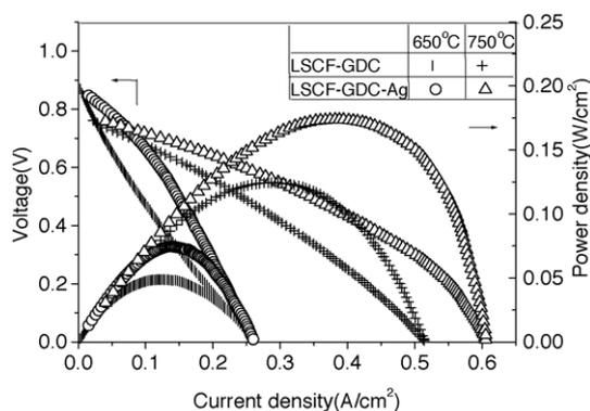
Fig. 5. The performance comparison of the SOFCs with LSCF-SDC and LSCF-SDC-Ag cathodes tested at 650 and 750 °C.
