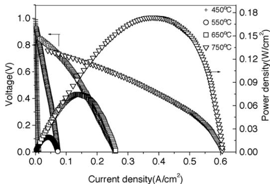
Fig. 4. The single SOFC performance with LSCF+SDC+Ag composite cathode at different temperatures.
