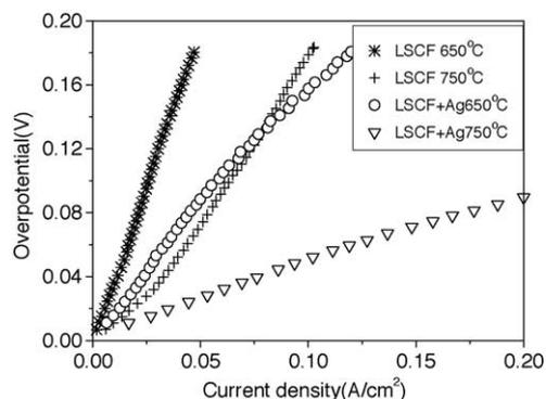
Fig. 3. Relations of overpotential and current density for different cathodes on the SDC electrolytes measured at 650 and 750 °C.
