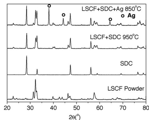
Fig. 1. The X-ray diffraction patterns of the SDC, LSCF powders and the sintered composite cathodes.
