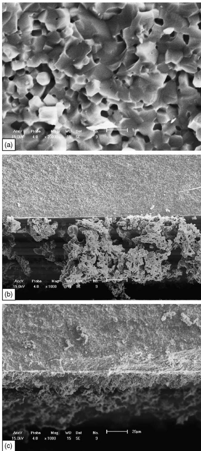
Fig. 2. SEM images of the SDC electrolyte (a), the cathode–electrolyte interfaces of LSCF–SDC/SDC (b) and LSCF–SDC–Ag/SDC (c).
