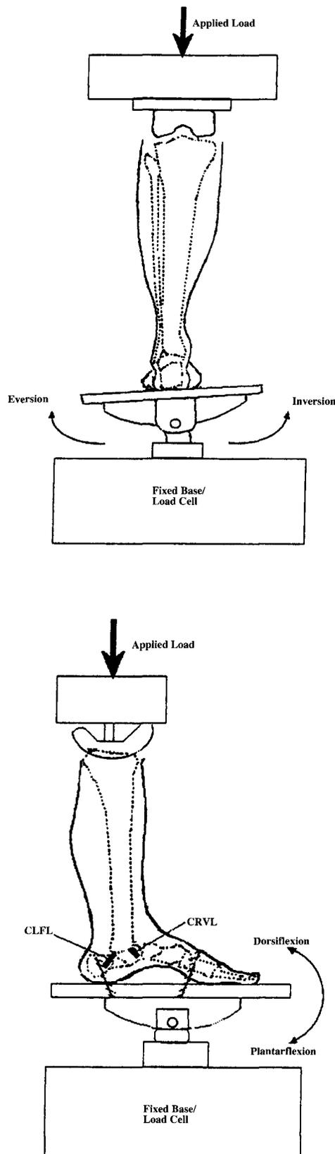
**Fig. 2:** Schematic of mechanical loading of experimental specimen. A 220N compressive load was applied to the upper tibial plateau via a metallic femoral knee component. A compound angle vise provided the ability to position and fix the foot in eversion/inversion and plantar/dorsiflexion. (a) Posterior view, (b) Medial view. CRVL - Cervical ligament; CLFL - Calcaneofibular ligament
